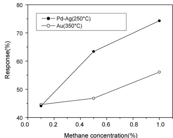
Fig. 6. Response as a function of methane concentration.
