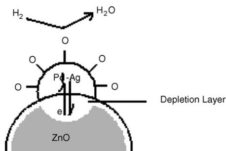
Fig. 9. Sensitization mechanism of Pd-Ag/ZnO sensor.
