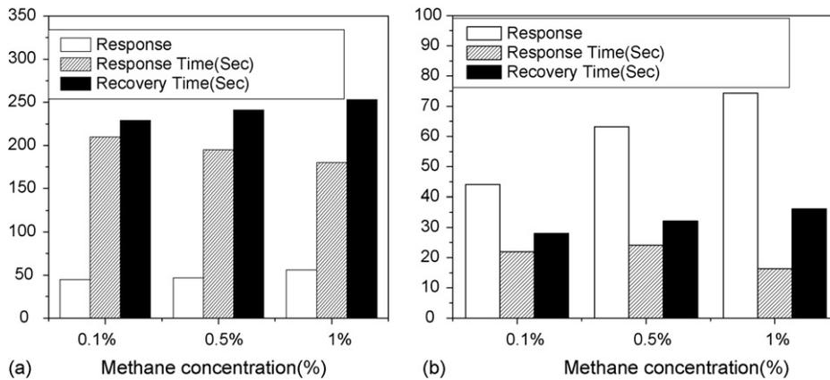
Fig. 8. Response, response time and recovery time as a function of gas concentration for (a) Au contact (350 °C) and (b) Pd-Ag (26%) contact (250 °C).
