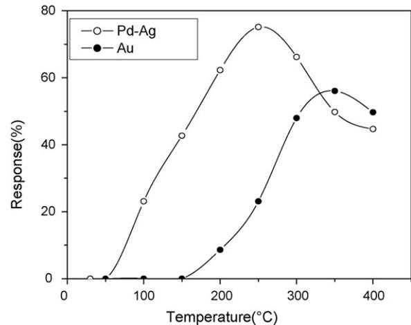
Fig. 5. Response to 1% methane as a function of temperature.
