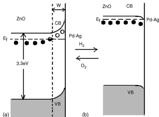
Fig. 10. Schematic band diagrams of Pd-Ag/ZnO in (a) oxidized state and (b) reduced state.
