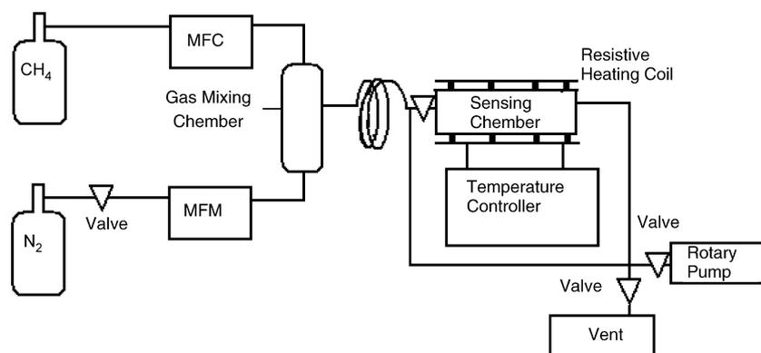
Fig. 2. Schematic of the gas sensor measurement setup.
