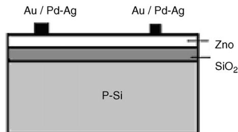
Fig. 1. Schematic of the sensor structure with an Au or Pd-Ag (26%) contact.
