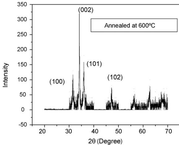
Fig. 3. The XRD pattern of the nanocrystalline ZnO surface annealed at 600 °C for 30 min.
