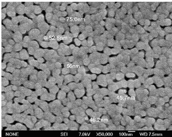
Fig. 4. SEM images of the nanocrystalline ZnO surface annealed at 600 °C for 30 min.
