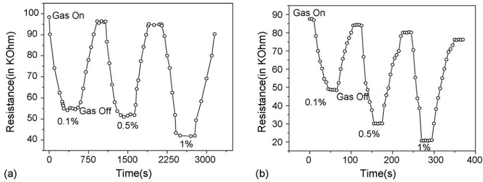
Fig. 7. Transient response characteristics with (a) Au contact (b) Pd-Ag contact.
