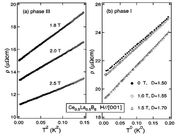
FIG. 2. The electrical resistivity of  $\text{Ce}_{0.5}\text{La}_{0.5}\text{B}_6$  (a) in phase III and (b) in phase I shown as a function of (a)  $T^2$  and (b)  $T^D$ . The field and current are directed along the [001] and  $[1\bar{1}0]$  axes, respectively. Solid lines are fits.
