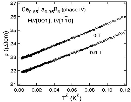
FIG. 6. The electrical resistivity of  $\text{Ce}_{0.65}\text{La}_{0.35}\text{B}_6$  in phase IV shown as a function of  $T^2$ . The fields and current are directed along the [001] and  $[1\bar{1}0]$  axes, respectively. The solid lines are fits.
