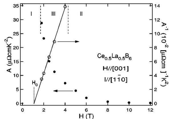
FIG. 3. The coefficients  $A$  (solid circles) of the  $T^2$  term in the resistivity of  $\text{Ce}_{0.5}\text{La}_{0.5}\text{B}_6$  shown as a function of magnetic field. The field and current are directed along the [001] and  $[1\bar{1}0]$  axes, respectively. This figure includes  $A^{-1}$  (open circles) in phase III. The solid line is a fit to  $A^{-1}$ .
