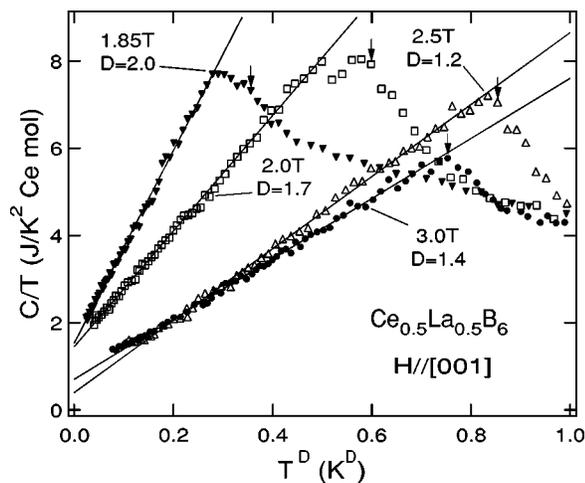
FIG. 5. The specific heat over temperature of  $\text{Ce}_{0.5}\text{La}_{0.5}\text{B}_6$  per Ce mole as a function of  $T^D$ . The arrows indicate the phase I–phase III or phase II–phase III transition points and this system is in phase III at low temperatures. Solid lines are fits by the formula  $C/T = \gamma + \beta T^D$ .
