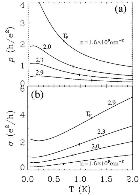
FIG. 3. Calculated (a) resistivities and (b) conductivities for  $n$ -GaAs system for various electron densities  $n = 1.6, 2.0, 2.3, 2.9 \times 10^9 \text{ cm}^{-2}$  with the remote charged impurities and a fixed Dingle temperature  $T_D = 0.75 \text{ K}$  as a function of temperature. The vertical bars indicate the Fermi temperature  $T_F$ .
