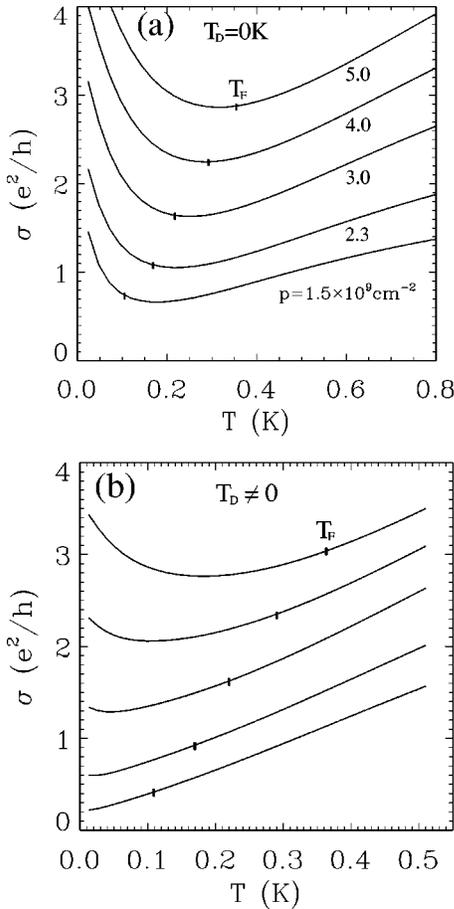
FIG. 2. Calculated conductivities for  $p$ -GaAs system (Ref. 7) for various hole densities  $p = 5.0, 4.0, 3.0, 2.3, 1.5 \times 10^9 \text{ cm}^{-2}$  (from the top) with the remote charged impurities. In (a) we calculate conductivities without level broadening in the polarizability function, and in (b) we include the level broadening in the screening, following Ref. 4, with  $T_D = 0.2, 0.25, 0.3, 0.4, 0.5 \text{ K}$  (from the top). The vertical bars indicate the Fermi temperature  $T_F$ .
