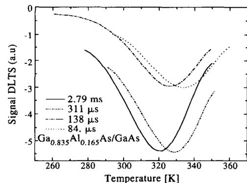
Figure 4. DLTS signal for different widths of filling pulse. Measuring parameters:  $f = 12.7\text{Hz}$ ,  $U_1 = -6\text{V}$ ,  $U_2 = -8\text{V}$ ,  $U_R = -10\text{V}$ .
