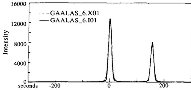
Figure 1. Reflectivity vs scan angle for the  $\text{Ga}_{0.560}\text{Al}_{0.440}\text{As}/\text{GaAs}$  sample.  $\cdots$  measured reflectivity curve for the sample under study,  $\text{—}$  simulated reflectivity curve with a lattice misfit data of 1133 ppm.
