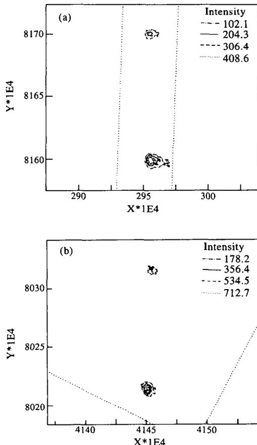
Figure 2. The map of reciprocal lattice points for  $\text{Ga}_{0.560}\text{Al}_{0.440}\text{As}/\text{GaAs}$  sample. (a) Symmetrical reflex (006), (b) asymmetric reflex (226). The plot is in units  $\lambda/2d_{hkl}$ .
