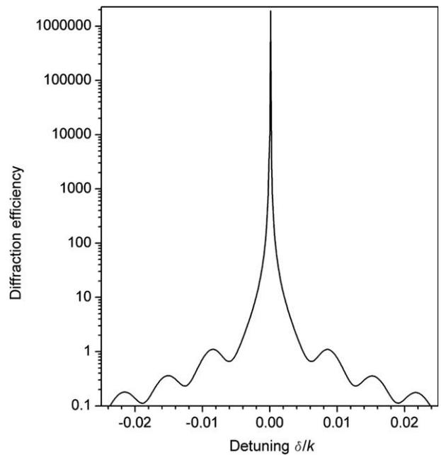
Fig. 4. Calculated pre-oscillations diffraction efficiency contour for a gain grating. The grating parameters are  $\alpha/k = 10^{-3}$ ,  $\kappa_n = 0$ ,  $\kappa_\alpha = 1.05 \times 10^{-3}$ ,  $d = 1000/k$ . Note the logarithmic scale.
