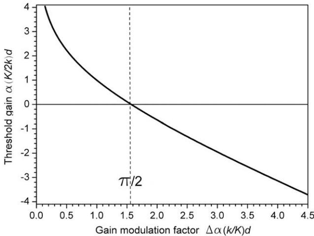
Fig. 5. Calculated threshold gain  $\alpha(K/2kd)$  as a function of the modulation factor  $\Delta\alpha d/2\sin\theta_B$  for a pure gain grating.
