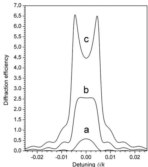
**Fig. 2.** Diffraction efficiency contours calculated for pure phase grating with uniform gain. (a) Zero gain,  $\Delta n/n = 1.8 \times 10^{-3}$ . (b) The same contour calculated with the presence of the uniform gain  $\alpha/k = 8 \times 10^{-4}$ . (c) The same with  $\alpha/k = 1.1 \times 10^{-3}$ .
