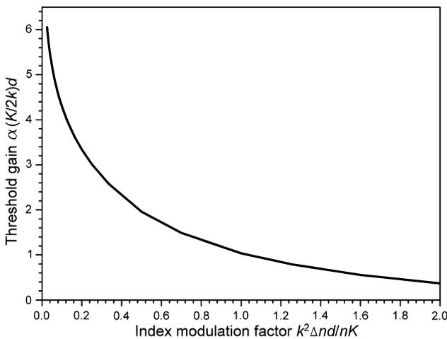
Fig. 6. Calculated threshold gain  $\alpha(K/2kd)$  as a function of the modulation factor  $k^2\Delta n d/nK=k\Delta n d/2\sin\theta_B$  for a pure phase grating with uniform gain.
