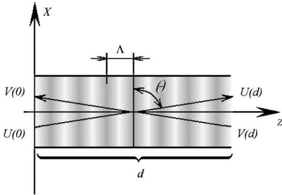
**Fig. 1.** Schematic of the waves in the modulated medium:  $U$  is the incident wave,  $V$  is the diffracted wave,  $\theta$  is the propagation angle,  $\Lambda$  is the grating spacing,  $d$  is the thickness of the grating.
