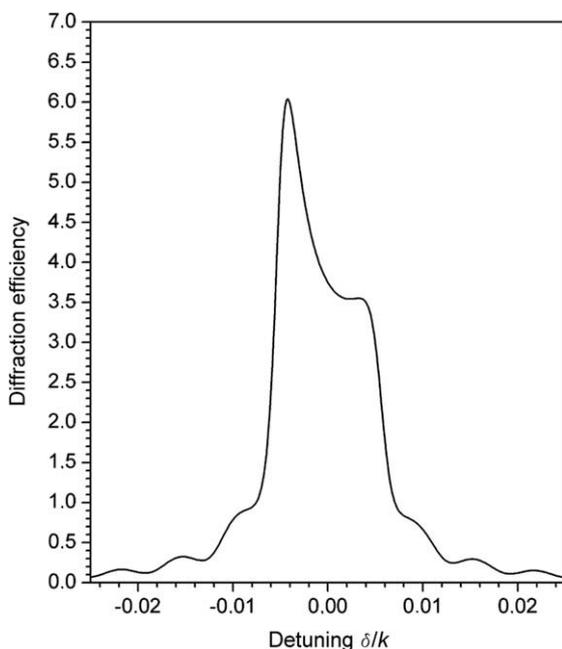
Fig. 3. Diffraction efficiency contour calculated for mixed-type grating with gain  $\alpha/k = 10^{-3}$ ,  $\kappa_n = 10^{-3}$ ,  $\kappa_\alpha = 10^{-4}$ ,  $d = 1000/k$ .
