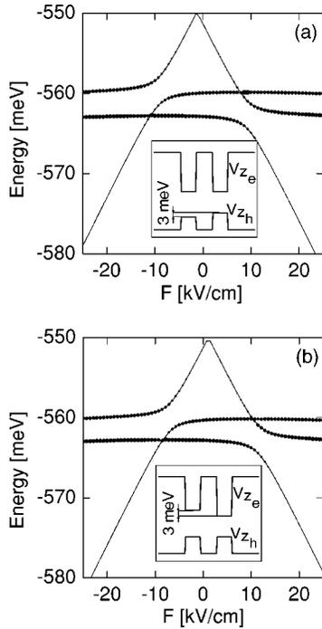
FIG. 4. Stark effect for the asymmetric system of quantum dots at  $b=6$  nm. In (a) the electron confinement is symmetric and the left dot for the hole is shallower by 3 meV. In (b) the hole confinement is symmetric and the left dot for the electron is shallower by 3 meV. The insets in (a) and (b) show a schematic drawing of the vertical confinement for  $F=0$ .
