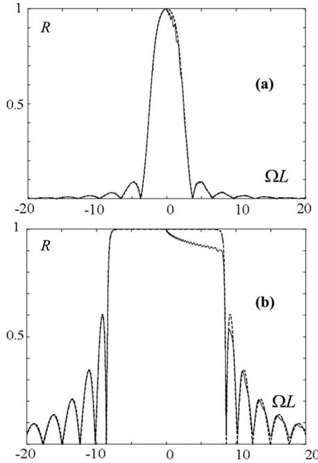
FIG. 2. Reflection coefficient vs frequency detuning calculated from simplified formula (9) (solid lines) and from full Eqs. (5) and (6) (dashed lines) at  $L=520$  ( $l=1.5$  cm). (a)  $\alpha=0.0025$  and (b)  $\alpha=0.01$ .
