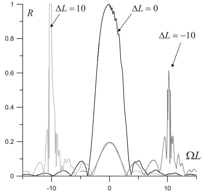
FIG. 3. The shift in the reflection zone when varying the mismatch parameter  $\Delta$ , which depends on distance between plates  $b_0$  at  $L=520$  and  $\alpha=0.0025$ .
