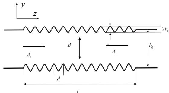
FIG. 1. Scheme of terahertz band Bragg reflector of planar geometry.
