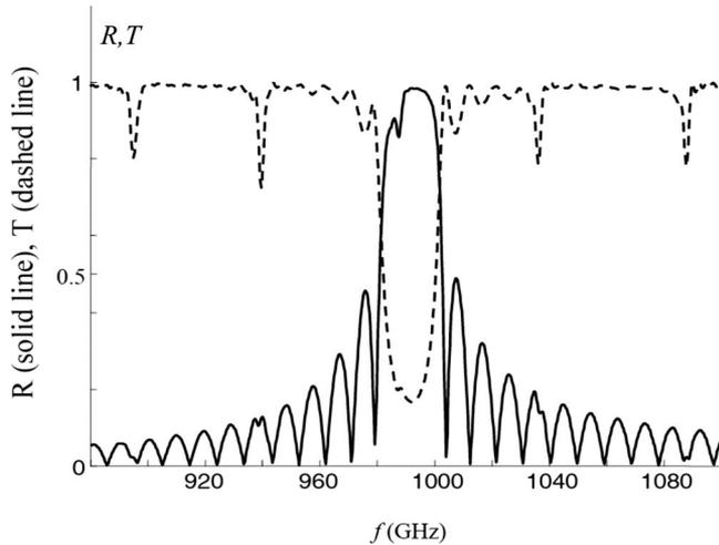
FIG. 4. Reflection (solid line) and transmission (dashed line) coefficients vs frequency found in 3D simulations at  $b_0=0.6$  cm,  $d=0.03$  cm,  $b_1=0.003$  cm, and  $l=1.5$  cm.
