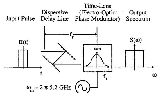
FIG. 1. Experimental schematic of the time-to-frequency converter with the ideal time lens approximated by a sinusoidally driven, electro-optic phase modulator.
