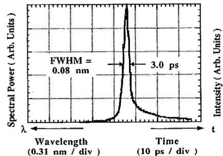
FIG. 3. Measured system time resolution found by performing time-to-frequency conversion on a pulse whose autocorrelation width is 1.9 ps.
