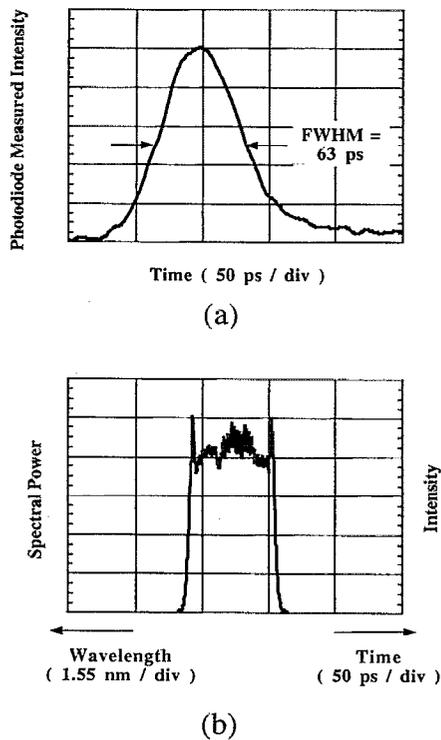
FIG. 4. Effect of aberrations on long pulses. (a) Photodiode measured input pulse. (b) Pulse shape measured with new technique shows aberrations due to overfilling the time-lens aperture.
