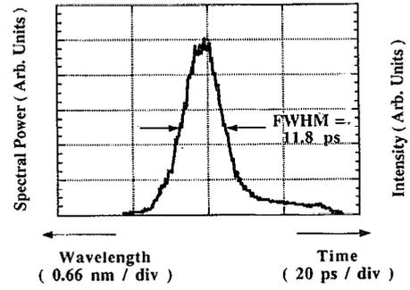
FIG. 2. Pulse shape measured by time-to-frequency conversion.
