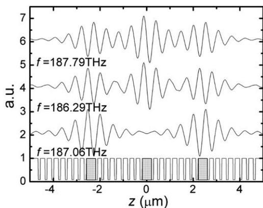
Fig. 6. Electric field and the refractive index distribution in the third order PC filter at  $N_{\text{outer}} = 7$  and  $N_{\text{inner}} = 7$ . Two anti-symmetrical modes  $f = 186.29, 187.79$  THz and one symmetrical mode  $f = 187.06$  THz are shown.
