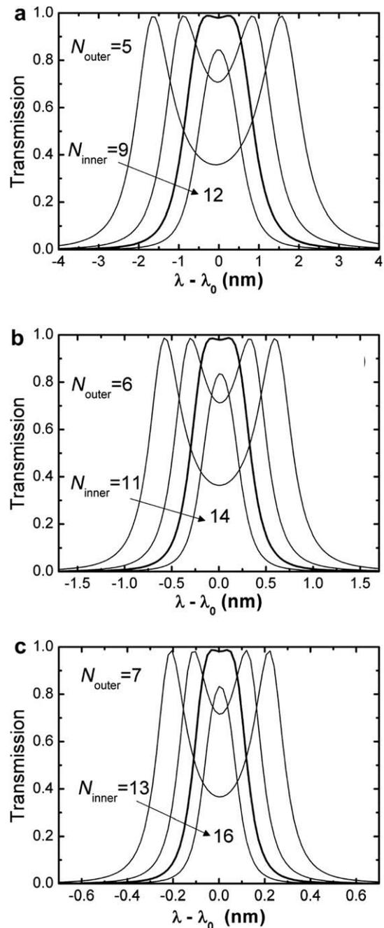
Fig. 2. Spectra responses of second order PC filters with tapers. (a)  $N_{\text{outer}} = 5$  (including the tapers), (b)  $N_{\text{outer}} = 6$ , (c)  $N_{\text{outer}} = 7$ . The spectra at  $N_{\text{inner}} = 2, N_{\text{outer}} + 1$ , i.e.  $k = 1$ , are plotted as thick solid lines.
