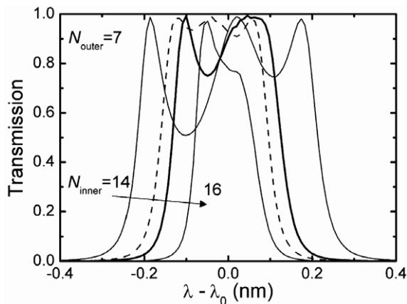
Fig. 5. Spectra responses of third order PC filters with tapers, where  $N_{\text{outer}} = 7$  and  $N_{\text{inner}}$  varies from 14 to 16. The response in an optimized third order filter is shown as dashed line.
