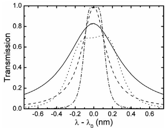
**Fig. 4.** Spectra responses in a single cavity PC filter without (solid line) and with (dashed line) tapers, and in the corresponding second order filters without (dotted line) and with (dash dot) tapers, where  $N_{\text{outer}} = 7$ .
