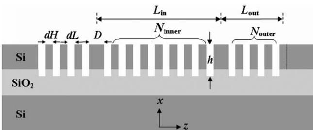
Fig. 1. Schematic of a second order 1D PC filter on SOI material ( $N_{\text{inner}} = 7$ ,  $N_{\text{outer}} = 3$ ).
