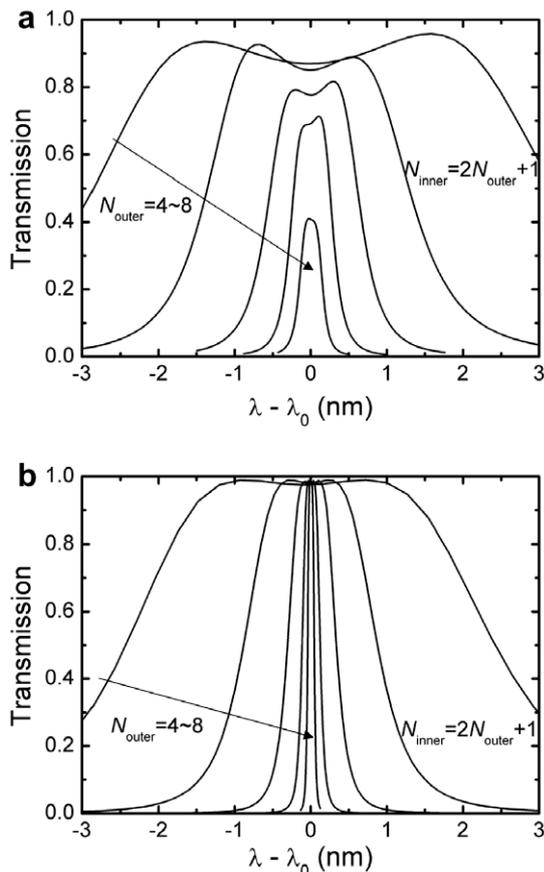
**Fig. 3.** (a) Spectra responses of second order PC filters without tapers. (b) Spectra responses of second order PC filters with tapers. In both cases,  $N_{\text{inner}} = 2, N_{\text{outer}} + 1$ , i.e.  $k = 1$ , and  $N_{\text{outer}}$  varies from 4 to 8.
