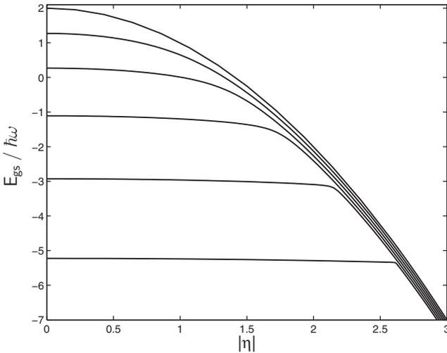
FIG. 2. Ground-state energy as a function of the dimensionless electric field  $\eta$ , for various values of the Coulomb interaction  $E_C$ , calculated as the solid line of Fig. 1. From top to bottom  $E_C$  varies from 0 to 2.5 in steps of 0.5. For larger  $E_C$  one can more clearly distinguish a plateau (due to dominating Coulomb interaction) from the nearly free regime.
