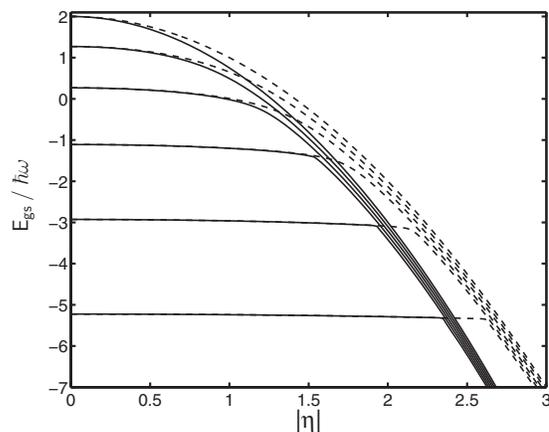
FIG. 6. Ground-state energy as a function of the dimensionless electric field  $\eta$  for different confinement energies (solid) and equal confinement energies (dashed). From top to bottom the relative strength of the Coulomb interaction  $E_C$  varies from 0 to 2.5 in steps of 0.5. For different confinement energies the transition point occurs at smaller fields.
