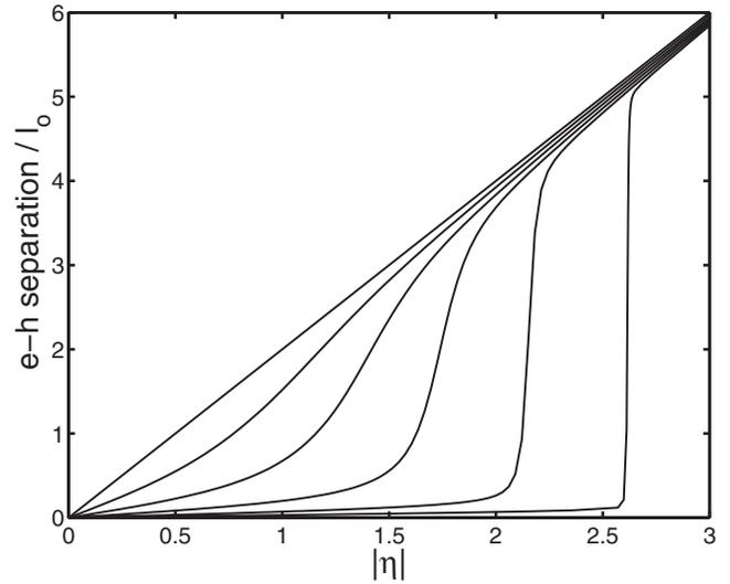
FIG. 3. Separation of electron and hole as a function of the dimensionless applied field  $\eta$  for different values of the relative strength of the Coulomb interaction  $E_C$ . From left to right:  $E_C$  varies from 0 to 2.5 in steps of 0.5. For larger values of  $E_C$  the transition point occurs only for higher electric fields and the transition becomes more abrupt.
