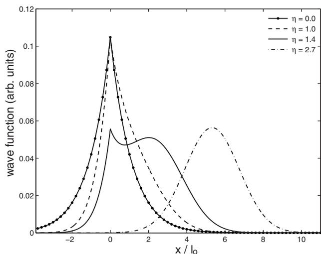
FIG. 5. Cross section of the ground-state wave function for  $E_C=1$  and different values of the applied bias. A transition from the Coulomb dominated state for small fields to the shifted harmonic oscillator state for large fields can be observed.
