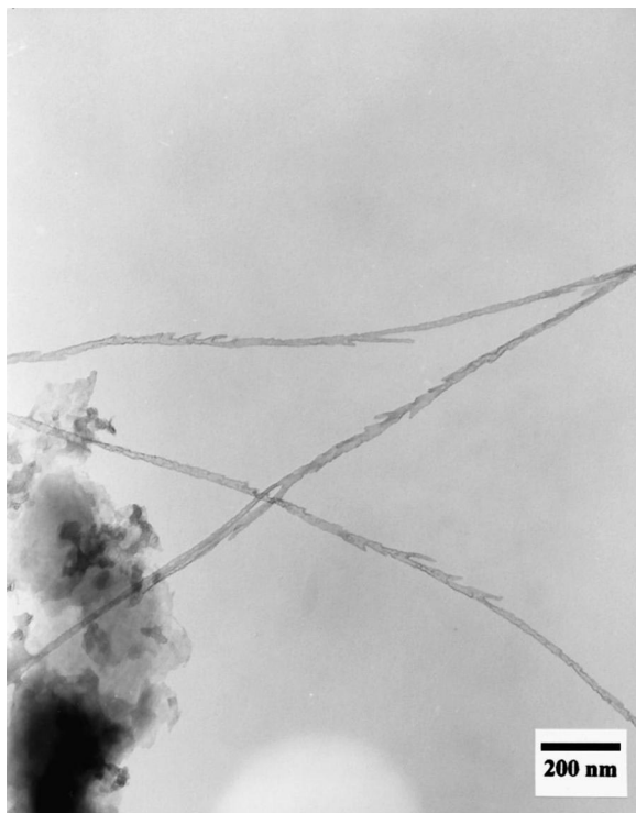
Fig. 5. TEM images of CNTs grown at 550°C by CVD in templates anodized at 18 V in 1.2 M sulfuric acid solution.
