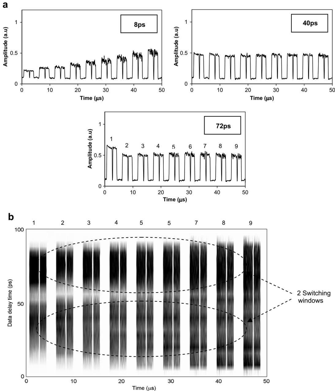
**Fig. 6.** Memory performance as a function of delay in the data. (a) variation in data pulse timings for the two optimum positions for each window of 40 ps and 72 ps and a less efficient operating position of 8 ps showing in all cases recovery to a stabilised level. (b) Full sweep of variation in input timings showing the two switching windows expected from a symmetrical SOA offset.
