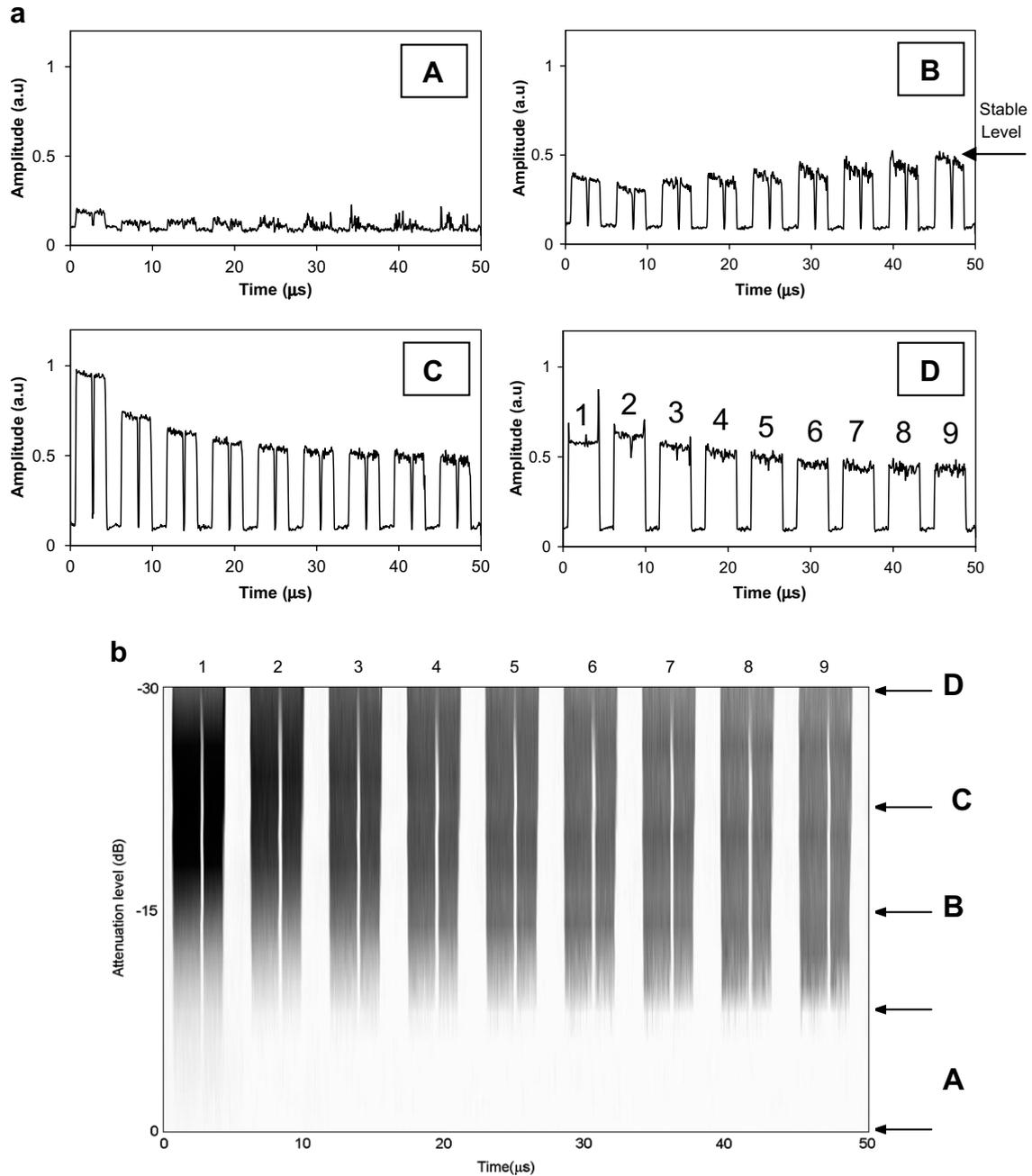
**Fig. 5.** Characterisation of the first nine circulations: (a) data stored recovering to a stabilised level, for changing input data powers and (b) the full range of varying initial data input powers, starting from where the initial data is too low and no data is stored, A, increasing to B and C where good contrast between the zero and one levels is maintained and finally the initial data packet power is high enough to cause the zeros to become ones thus corrupting the data, at D.
