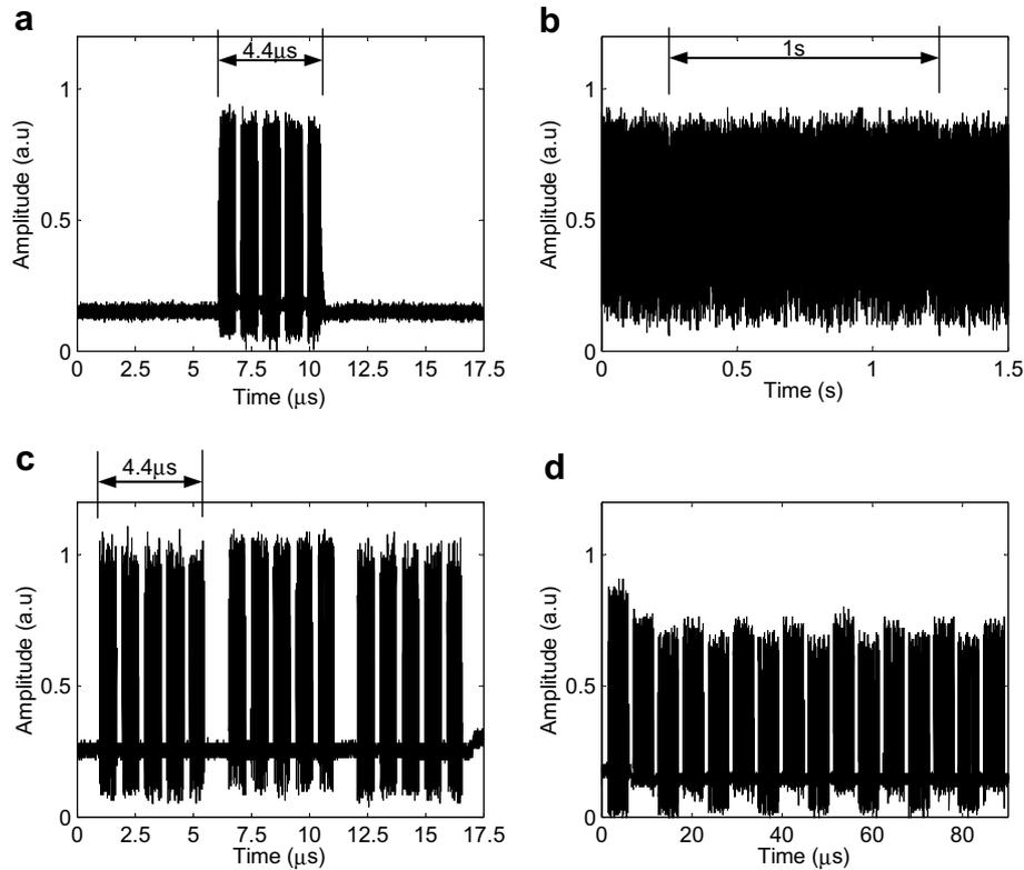
**Fig. 3.** Experimental traces showing the memory function (a) the initial data packet consisting of 44 kbs of data (equivalent to 4.4 μs), (b) data is stored for 1 s, (c) the final three blocks of stored data after 1 s of storage time (d) the initial 15 circulations of data storage demonstrating the self-leveilling transient of the device.
