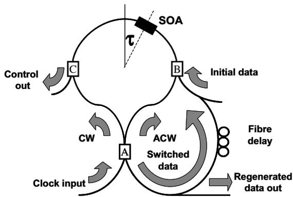
**Fig. 1.** Schematic diagram of the optical memory. The clock input is used to inject a continuous supply of fresh pulses to the optical switch. The Initial data input is used to load the memory.
