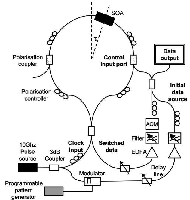
**Fig. 2.** Experimental setup, a fibre ring laser provides 10 GHz pulse streams for both the clock and the original data thus operating at the same wavelength. Before fresh data is stored the device is reset by disconnecting the feedback using an acousto-optical modulator (AOM). The data output is located at the end of the feedback just before the data re-enters the TOAD.
