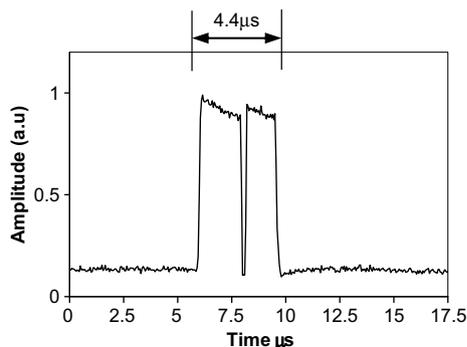
**Fig. 4.** Initial data pattern consisting of two blocks of 1 s separated by one block of 0 s. The total packet length used was 4.4 μs.
