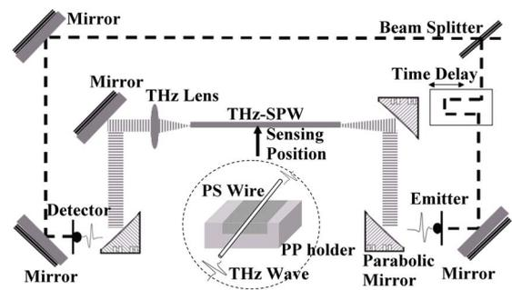
FIG. 1. (Color online) THz time-domain spectrometer based on subwavelength-diameter plastic wire (SPW). Inset shows THz pulse on an SPW propagated through powder materials in the PP channel.
