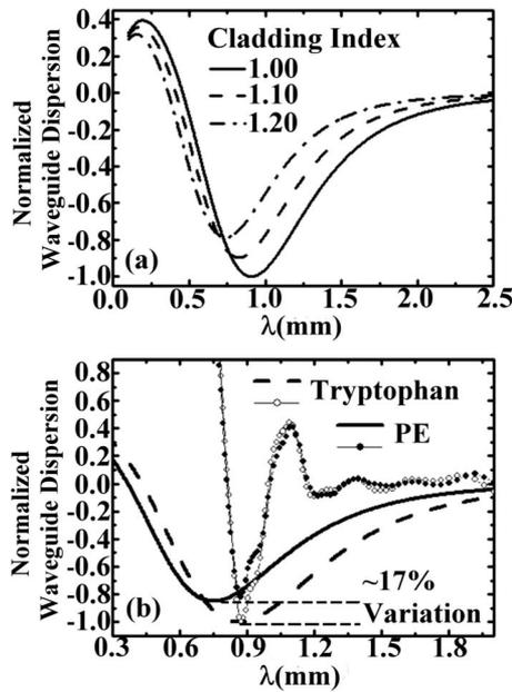
FIG. 3. (a) Theoretical normalized waveguide dispersions of 300  $\mu\text{m}$  thick PS wire with various cladding indices. (b) Measured (solid and dashed lines) and simulated (solid and open circles) waveguide dispersions of PS wire with PE and tryptophan powders in wire cladding regions.
