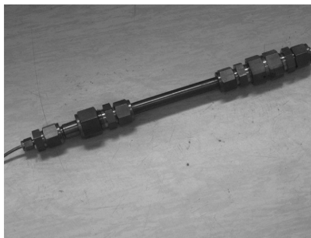
Fig. 1 – The assembled stainless steel reactor used for all OMCVD experiments; the main body sits within the furnace, whilst some of the evacuation line remains outside the furnace to prevent damage to the ball valve.
