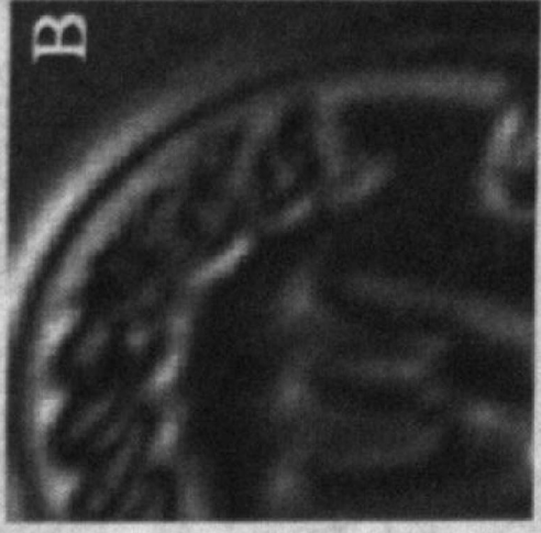
Fig. 3. A, B, D, Terahertz images and, C, visible-light photograph of a plastic coin. Left, transmitted terahertz power measured, A, parallel and, B, perpendicular to the original polarization direction (white is maximum transmission). C, Visible-light photograph of the coin. D, Plot of the angular rotation of the direction of the terahertz electric field (white is 0^\circ rotation, black is 45^\circ rotation).
