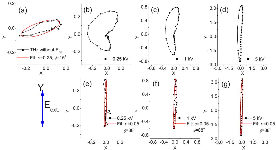
FIG. 1. (Color online) Polarization of terahertz emission from a filament with a dc field of (a) 0, (b) 0.25, (c) 1, and (d) 5 kV/cm. Terahertz polarizations in [(e)–(g)] were obtained at 0.25, 1, and 5 kV/cm by subtracting the waveforms without dc field, respectively.
