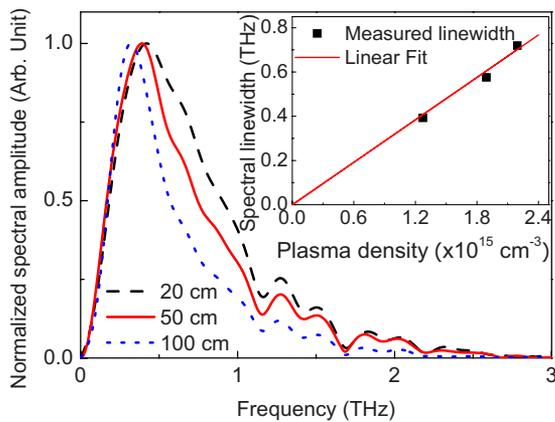
FIG. 4. (Color online) Normalized spectral amplitudes for linearly polarized terahertz emission from dc-biased filaments with 20 cm (dashed line), 50 cm (solid line), and 100 cm (dot line) focal length lens.  $E_{\text{ext}}=5$  kV/cm. The pump is 1.6 mJ. Inset: linear dependence between linewidth and plasma density.
