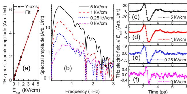
FIG. 2. (Color online) (a) Peak-to-peak amplitude of terahertz  $Y$  component as a function of external electric field. (b) Terahertz spectral amplitudes obtained by Fourier transforms with  $E_{\text{ext}}$  of 0 kV/cm (dashed-dot line), 0.25 kV/cm (dot line), 1 kV/cm (dashed line), and 5 kV/cm (solid line). Terahertz waveforms ( $Y$  axis) obtained with  $E_{\text{ext}}$  of (c) 5, (d) 1, (e) 0.25, and (f) 0 kV/cm. The pump was 1.6 mJ.
