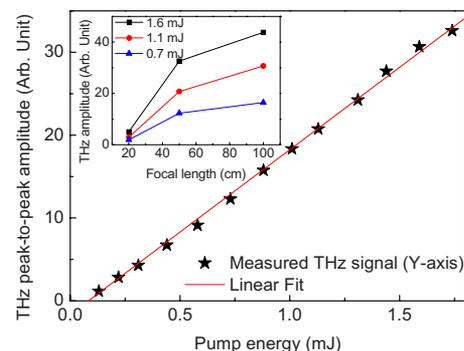
FIG. 3. (Color online) Peak-to-peak amplitude of the terahertz signal ( $Y$  axis) as a function of the pump energy with  $E_{\text{ext}} = 5$  kV/cm: experimental data (pentagons) and a linear fit (line), with 50 cm focal length lens. Inset: comparison of terahertz amplitudes ( $Y$  axis) from a dc-biased (5 kV/cm) filament formed by three focal length lens (20, 50, and 100 cm) when the pump energy is 0.7 mJ (triangles), 1.1 mJ (circles), and 1.6 mJ (squares).
