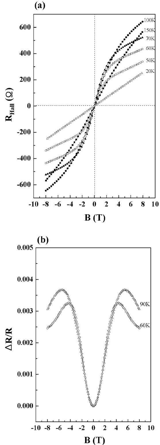
FIG. 3. (a) Hall resistance  $R_{Hall}$  of sample 5 as a function of the magnetic field  $B$  and (b) magnetoresistance of sample 5 as a function of the magnetic field  $B$  applied in the direction macroscopically parallel to the current.
