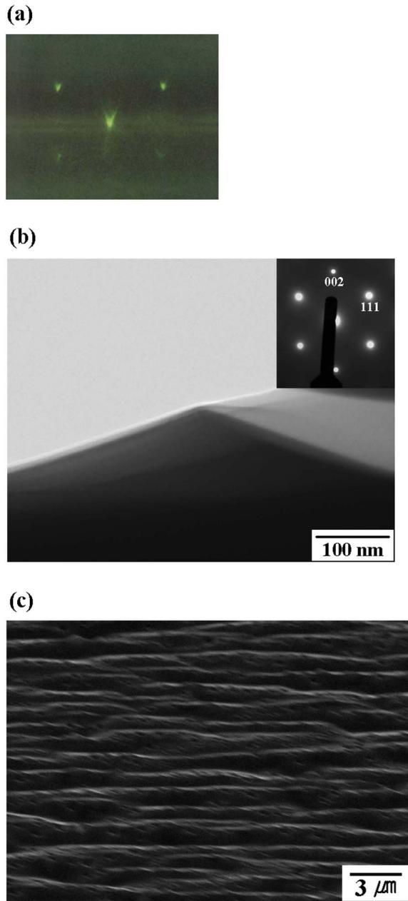
FIG. 4. (Color online) (a)  $[\bar{1}10]$  RHEED pattern for a GaAs buffer layer grown under a low As flux condition at  $0.98 \times 10^{-5}$  Torr and annealed for 5 min. (b) Cross-sectional TEM image of a faceted surface for sample 4 with a corresponding transmission electron diffraction pattern. (c) SEM image of the surface of sample 11.
