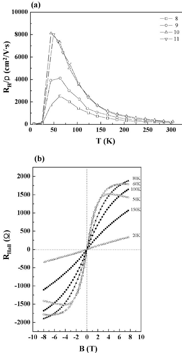
FIG. 5. (a) Plots of  $R_H/\rho$  as a function of the temperature  $T$  for samples 8–11. (b) Hall resistance  $R_{\text{Hall}}$  of sample 8 as a function of the magnetic field  $B$ .
