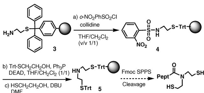
resin **3** was reacted with *o*-nitrobenzenesulfonyl chloride to afford the sulfonamide resin **4**. Alkylation of the sulfonamide with Trt-SCH<sub>2</sub>CH<sub>2</sub>OH by Mitsunobu reaction and subsequent thiolytic removal of the sulfonyl group yielded the desired dialkylamine resin **5**, ready for use in Fmoc SPPS.
