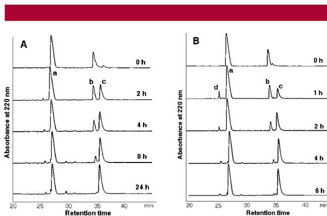
**Figure 2.** Ligation between H-LKSFG-BMEA and H-CLKFA-NH<sub>2</sub> in the presence of MESNa (2% w/v) and 50 mM TCEP and at pH 5. HPLC gradient: 0–50% buffer B in 50 min. (A) Reaction at 37 °C. (B) Reaction under microwave irradiation. Peak a, H-CLKFA-NH<sub>2</sub>; peak b, H-LKSFG-BMEA; peak c, ligation product; peak d, H-LKSFG-MES thioester.
