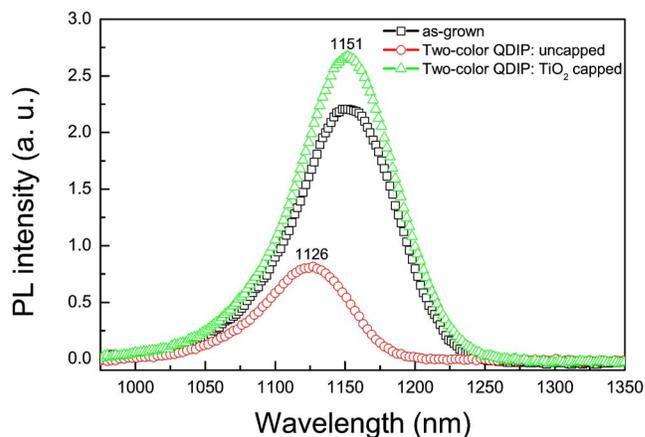
FIG. 1. (Color online) Room temperature PL spectra of the two-color QDIPs. The spectrum for the as-grown sample is also shown for comparison.
