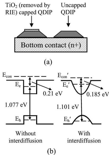
FIG. 2. (a) The schematic diagram of the two-color detector sample and (b) the band gap diagram showing various transitions within the two QDIPs.
