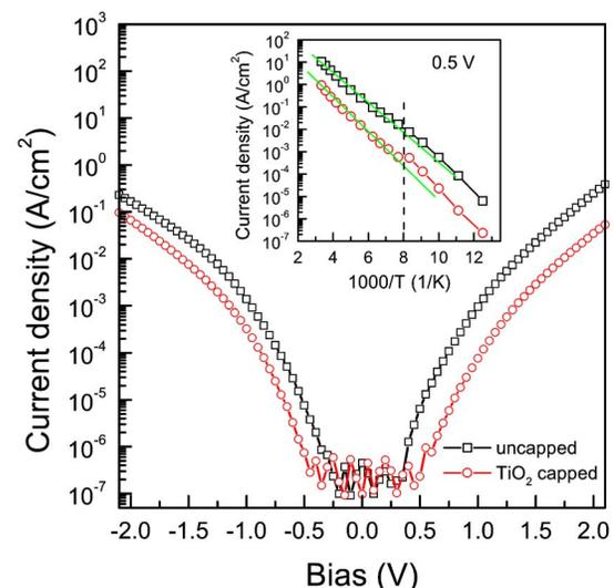
FIG. 4. (Color online) The 77 K  $I$ - $V$  characteristics of the two-color QDIPs. Inset plots the dark current density vs inverse temperature ( $1000/T$ ) at the bias of 0.5 V for both QDIPs.
