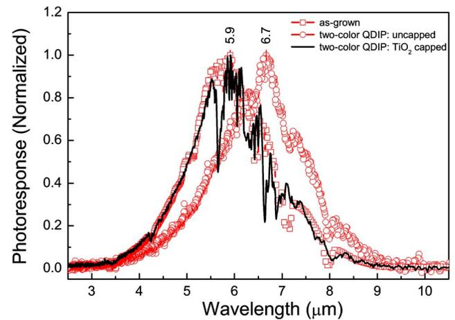
FIG. 3. (Color online) The 77 K spectral photoresponses of the two-color QDIPs, in comparison with the spectrum for the as-grown.
