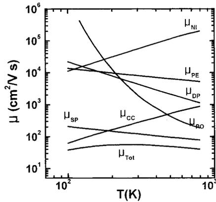
FIG. 3. Drift-mobility variations for various scattering mechanisms in interface layer (sample A).
