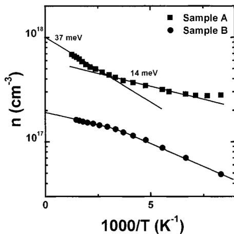
FIG. 4. Electron density variations as a function of inverse temperature.
