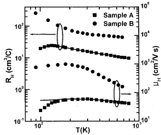
FIG. 2. Hall coefficient and Hall mobility measured as a function of temperature; A, interface layer; B, GaN layer.
