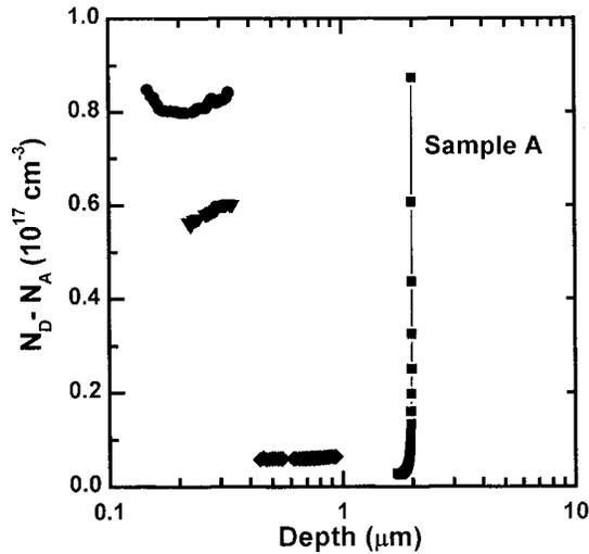
FIG. 1. Depth profile of  $C-V$  measurements for the samples of different electron density.
