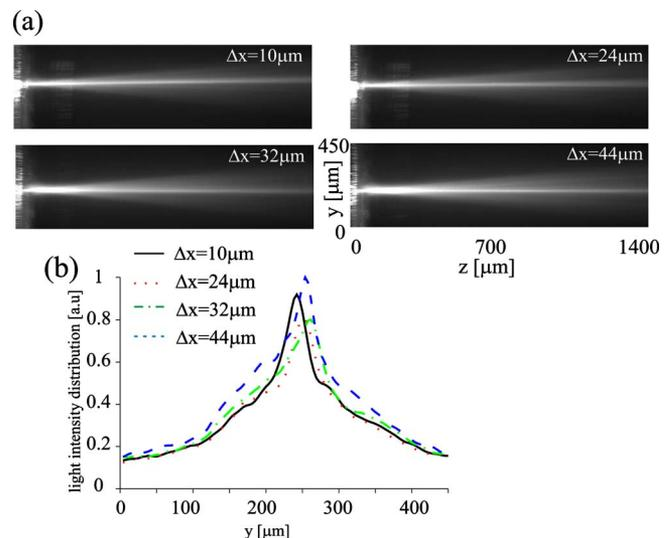
FIG. 4. (Color online) (a) Experimental results of creating spatial solitons in different layers across the ChNLC cell for different input vertical positions marked on photos as  $\Delta x$ . (b) Normalized intensity distribution profiles for each position and for the propagation distance  $\Delta z = 1000 \mu\text{m}$ .
