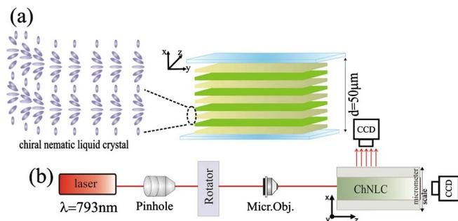
FIG. 1. (Color online) (a) Configuration of the analyzed NLC cell. (b) Schematic drawing of the experimental setup.
