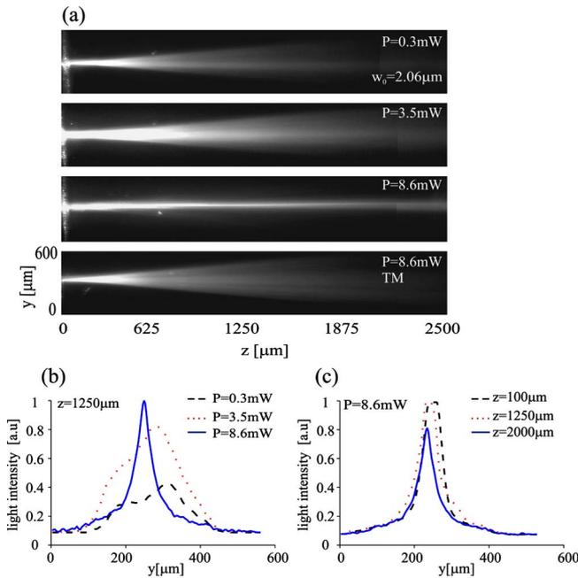
FIG. 2. (Color online) Experimental results of spatial solitons creation in ChNLCs layer for a Ti:sapphire laser: (a) light beam propagation for different inputs of light power (marked on photos) and centrally launching light beam, the last picture was taken for TM polarization. (b) and (c) Light intensity profiles for low and high power, respectively, and for different values of propagation distance.
