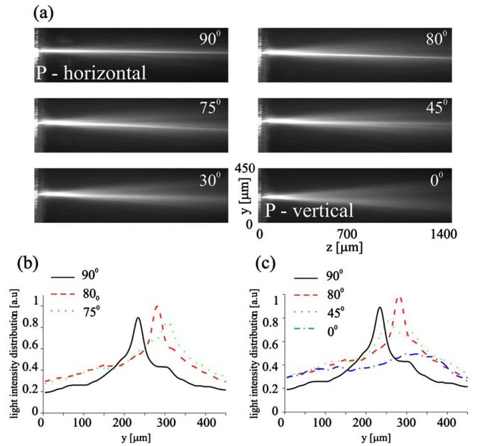
FIG. 3. (Color online) (a) Experimental results showing the beam walk-off effect by changing the polarization of input light beam. (b) Normalized light intensity profile distribution for three different polarizations for which the soliton changed its direction. (c) Normalized light intensity profiles for different polarizations crossing from TE to TM-like.
