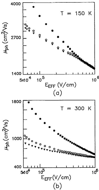
FIG. 3. Phonon-limited mobility of the electrons in a silicon-inversion layer vs the effective transverse-electric field. The effects of the number of subbands taken into account in the Monte Carlo simulation of parallel-electron transport is shown. (a) and (b) correspond to  $T=150$  K and  $T=300$  K, respectively. Data have been obtained by allowing the electrons to move in one subband (closed circles), three subbands (triangles), or six subbands (open circles).
