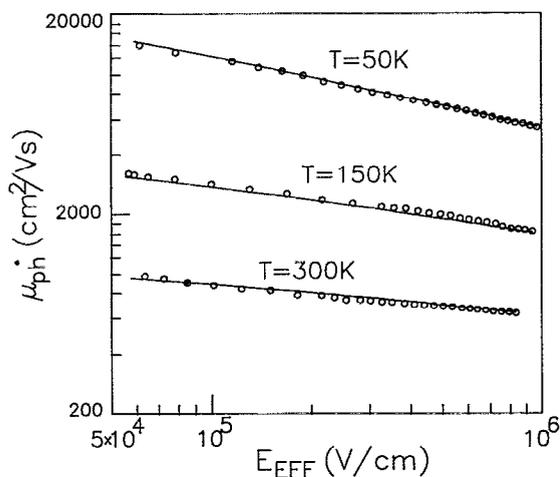
FIG. 5. Phonon-limited mobility of electrons in a silicon-inversion layer vs the effective-transverse-electric field obtained by a complete Monte Carlo simulation of the electron transport, at different temperatures (circles). Solid-line curves correspond to an empirical model based on an analytical expression. Excellent agreement can be noted.
