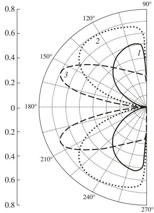
**Fig. 2.** Directional pattern of the terahertz radiation in the reflection of a laser pulse from a dense plasma ( $\omega_p \tau = 100$ )
