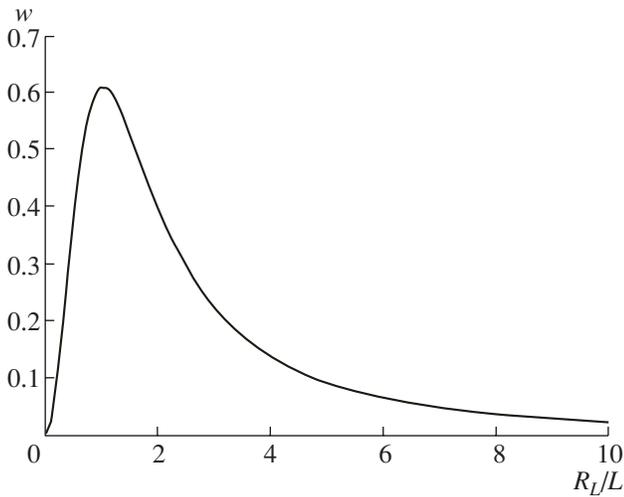
**Fig. 3.** Dimensionless total energy of the terahertz radiation from a laser pulse in its reflection from a dense plasma ( $\omega_p \tau = 100$ ) as a function of the radius-to-length ratio  $R/L$  of the pulse.
