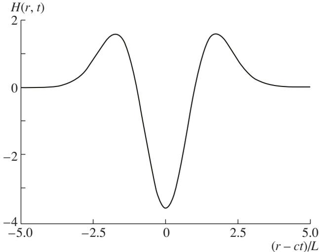
**Fig. 4.** Spatiotemporal distribution of the dimensionless magnetic field in a terahertz radiation pulse (5.4) generated in the reflection of a laser pulse (with  $R_L^2 = 2L^2$ ) propagating at the angle  $\theta = \pi/4$  from the boundary of a dense plasma ( $\omega_p \tau = 100$ ).
