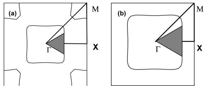
Fig. 2. Equi-frequency contours of TM (a) and TE (b) for frequency  $f = 0.26(c/a)$  of the PIS structure. The square with rounded corners centered  $\Gamma$ -point is the EFC of the second band; the curves centered M-point correspond to the third band of TM-polarized light. The shaded region shows the wide angle that self-collimation can be realized.
