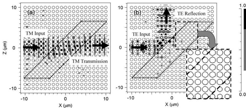
Fig. 4. Steady-state electrical field distribution for TM-polarized light (a) and magnetic field distribution for TE-polarized light (b) at frequency  $f = 0.27(c/a)$  calculated using the two-dimensional FDTD method. The inset in (b) shows the enlarged display of the polarization splitting part of the device with the radius  $R' = 1.2R$ .
