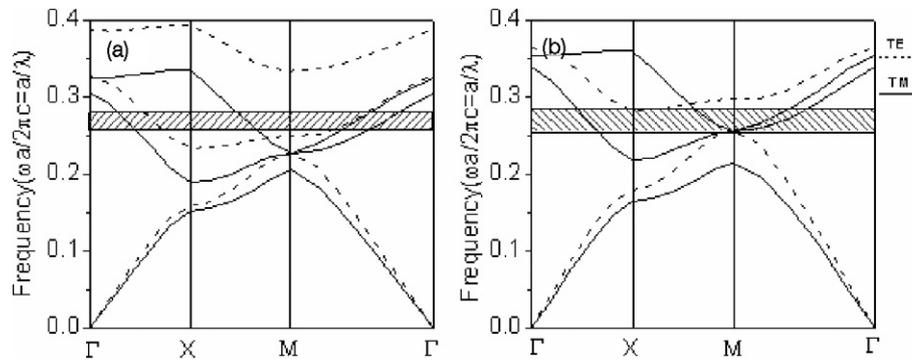
Fig. 3. Band diagrams of the PIS (a) and polarization splitting structure (b). The dot and solid lines represent the polarization bands of TE- and TM-polarized light, respectively. The shaded bar of (a) marks the polarization independent self-collimation frequencies  $f = 0.258\text{--}0.281(c/a)$ . The TE-polarized light band gap (shaded bar of (b)) appears to open at frequency  $f = 0.258\text{--}0.283(c/a)$ .
