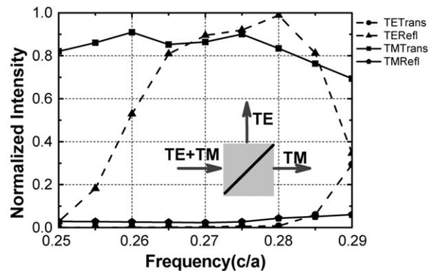
Fig. 5. Reflection efficiency and transmission efficiency versus frequency for TE- and TM-polarized light are shown. Dash line with triangular dots is corresponded to the TE-polarized light and solid line with square dots to the TM-polarized light. Schematic picture depicting the separation of TE- and TM-polarized light by the PBS is shown in the inset of the figure.
