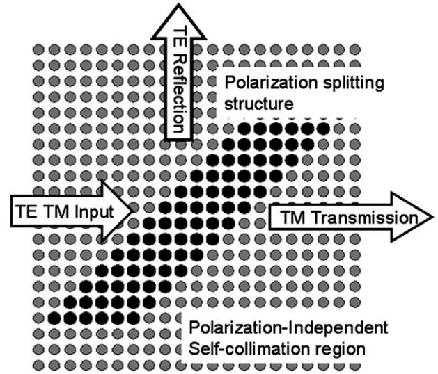
Fig. 1. Polarization beam splitter structure. The grey and black regions represent non-channel PIS structure and polarization splitting structure, respectively; the marked arrows indicate the propagation direction of TE- and TM-polarized light.
