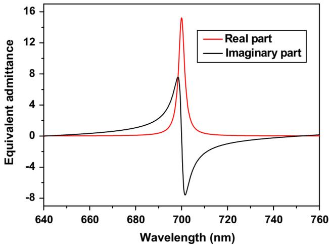
Fig. 1. Equivalent admittance of  $(LH)^22L(HL)^4/Sub$ .
