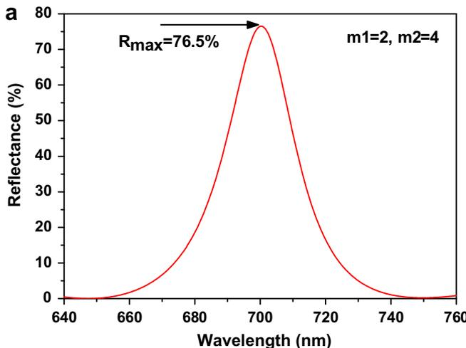
where  $Y = C'/B'$  and  $B', C'$  are, respectively matrix elements of the stack  $(LH)^{m1}2L(HL)^{m2}H/Sub$ . Thus, the reflectance at normal incidence of this filter can be calculated based on  $R = \frac{|B-C|^2}{|B+C|^2}$  [14] and  $B'$  will not affect the reflectance calculation:
