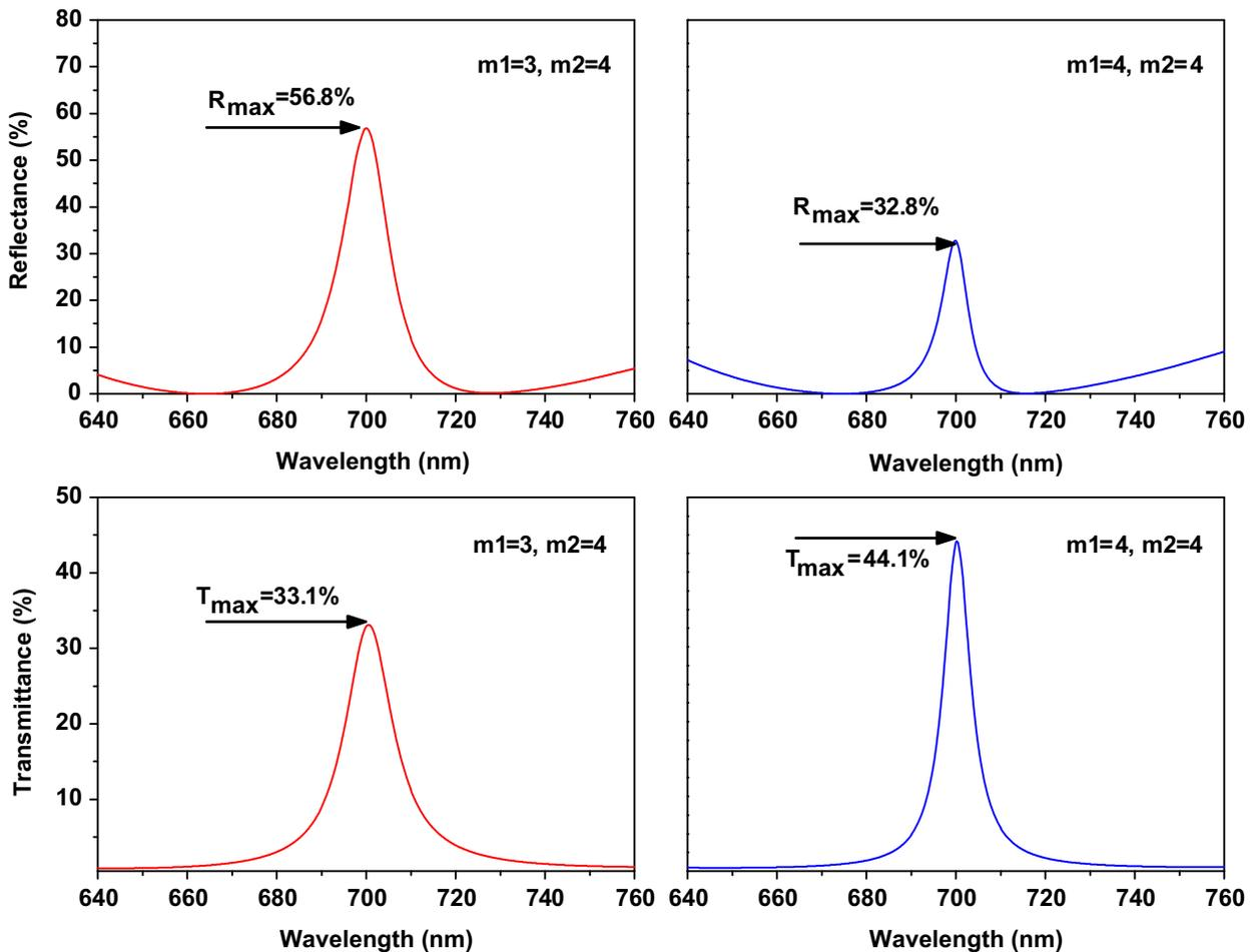
Fig. 4. The calculated transmittance and reflectance curves from 640 nm to 760 nm when  $m_1 = 3$ ,  $m_2 = 4$  and  $m_1 = 4$ ,  $m_2 = 4$ .
