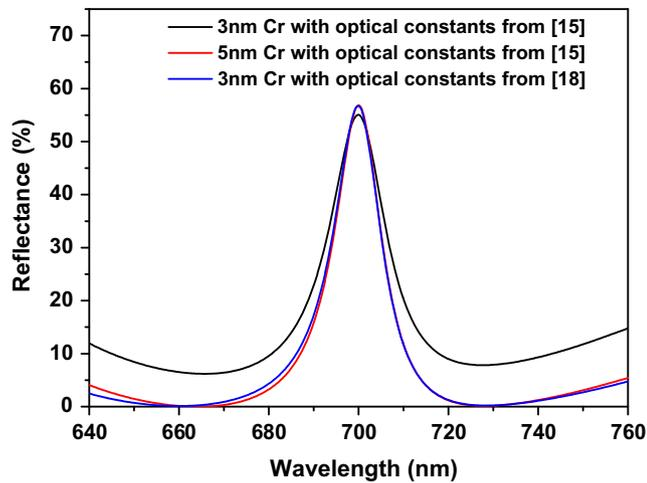
Fig. 6. The reflectance curves of the filter ( $m_1 = 3$ ,  $m_2 = 4$ ) with different optical constants of Cr film.
