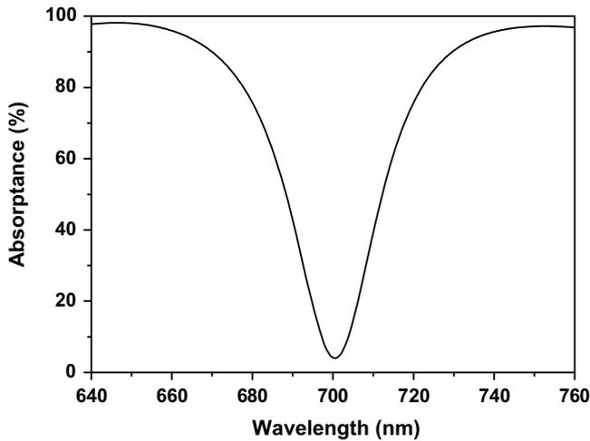
Fig. 3. The absorbance curve of Air/Cr  $(LH)^22L(HL)^4$ /Sub from 640 nm to 760 nm.
