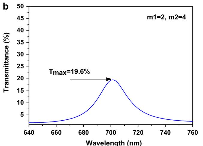
Fig. 2. The simulated results of Air/Cr  $(LH)^22L(HL)^4/Sub$  in the spectral range from 640 nm to 760 nm (a) the reflectance curve (b) the transmittance curve.
