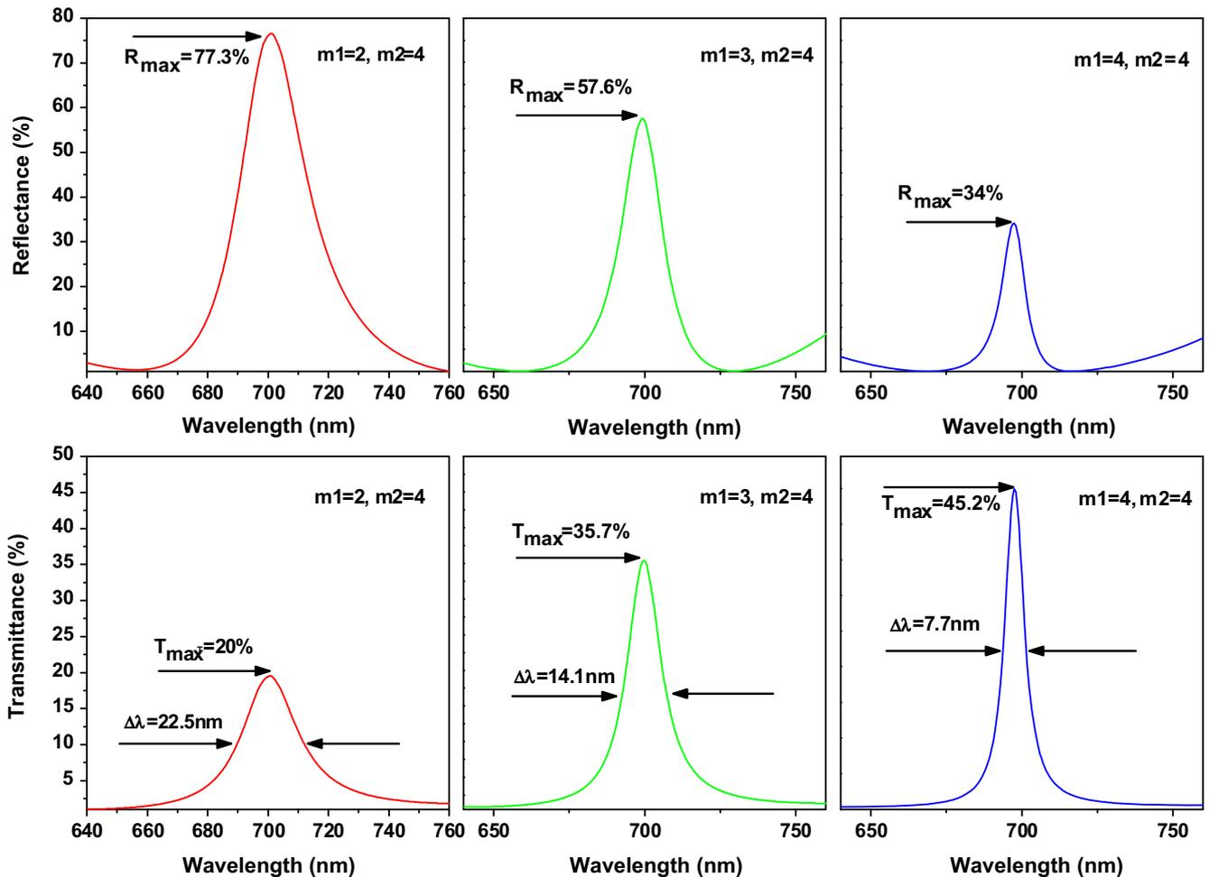
Fig. 5. The measured reflectance and transmittance curves in the spectral range from 640 to 760 nm at different  $m1$  values ( $m1 = 2-4$ ).
