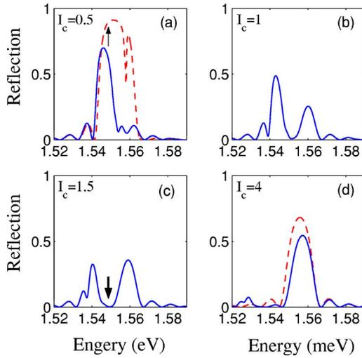
FIG. 2. (Color online) Reflection of the MQW system ( $N=150$ ) for various intensities of the control field ( $I_c$  in  $\text{MW}/\text{cm}^2$ ). The dashed line in (a) refers to the system's response when  $I_c=0$  and in (d) to the nonresonance PBG response of the structure in the absence of the excitons.
