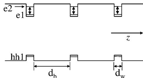
FIG. 1. Schematic diagram of the Bragg MQW structure interacting with an intense ir laser field.  $e1$  and  $e2$  refer to the conduction subbands and hh1 represents the heavy-hole subband. The two-sided arrows refer to the mixing processes caused by the ir laser.
