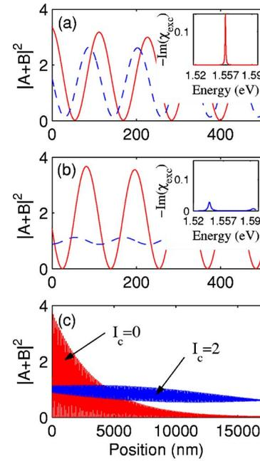
FIG. 3. (Color online) Total optical field inside the MQW structure for  $1.557$  (a) and  $1.549$  eV (b) and (c) when  $I_c=0$  (solid line) and  $2$   $\text{MW}/\text{cm}^2$  (dashed line). Insets of (a) and (b) show variation of imaginary parts of the susceptibility with  $I_c$ .  $A$  and  $B$  refer to the backward and forward waves.
