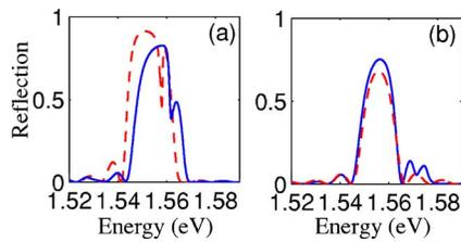
FIG. 4. (Color online) Reflection of the MQW ( $N=150$ ) for various  $I_c$  and  $\Delta_c = +20$  meV. The solid lines in (a) and (b) refer to  $I_c=0.5$  and  $2/\text{cm MW}/\text{cm}^2$ , respectively. Dashed line in (a) refers to the MQW response when  $I_c=0$  and in (b) to the nonresonant PBG in the absence of the exciton effects.
