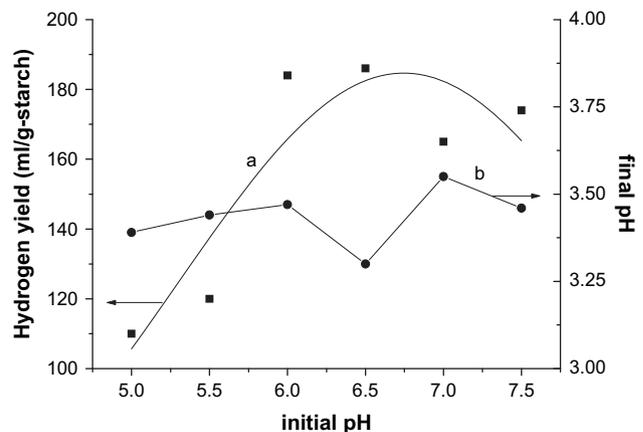
Fig. 1 – Hydrogen yield (curve a) (ml/g-starch) and final pH (curve b) versus initial pH at starch concentration 5 g/L with maximum hydrogen yield at pH 6.5.
