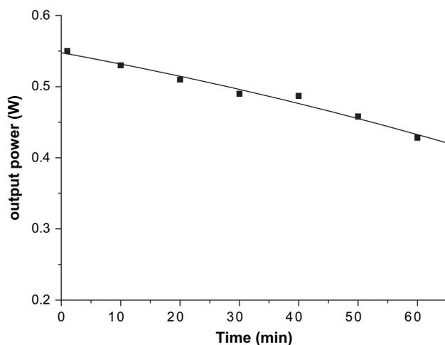
Fig. 4 – The time-output power profile generated by an in-house small PEMFC (2-cell stack, 10 cm<sup>2</sup>) through a 2 kΩ external loading fed with biogas.
