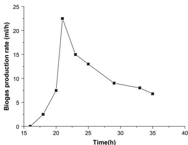
Fig. 3 – Biogas production rate versus biogas production time.
