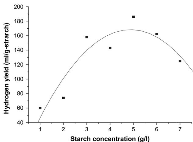
Fig. 2 – The correlation between hydrogen yield (ml/g-starch) and starch concentration at initial pH 6.5 with maximum hydrogen yield at starch concentration 5 g/L.
