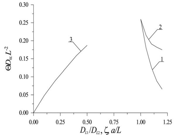
**Fig. 5.** Dependences of dimensionless compromise annealing time  $\vartheta = \Theta D_{0L} / L^2$  on some parameters of MS. Curve 1 is the dependence of  $\vartheta$  on the ratio  $D_{1L} / D_{2L}$  for  $\zeta = 0$  and  $a = L/2$ . Curve 2 is the dependence of  $\vartheta$  on the parameter  $\zeta$  for  $D_{1L} / D_{2L} = 1$  and  $a = L/2$ . Curve 3 is the dependency of the  $\vartheta$  on the ratio  $a/L$  for  $D_{1L} / D_{2L} = 1$  and  $\zeta = 0$ .
