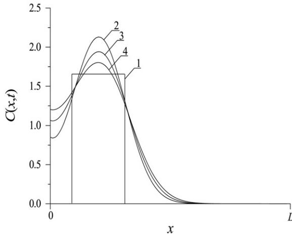
**Fig. 4.** Spatial distribution of dopant in MS for implanted-junction rectifier. Curve 1 is idealized spatial distribution of dopant. Curves 2–4 are spatial distributions of dopant for different values of annealing time (increasing of number of curves corresponds to increasing of value of annealing time).
