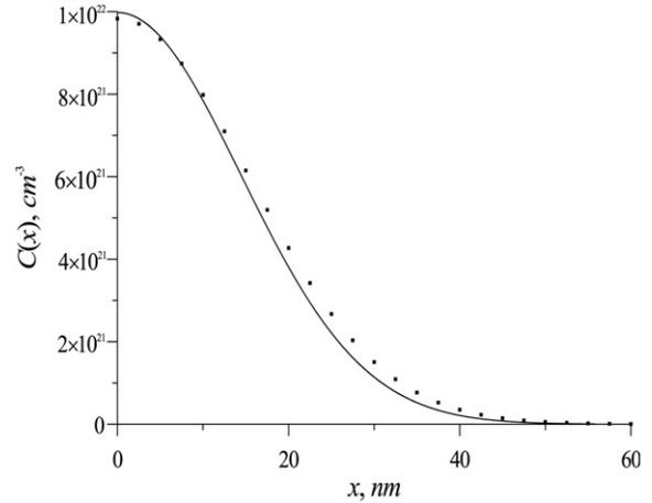
**Fig. 3.** Solid line is calculated distribution of dopant. Squares are experimental distribution of boron concentration in silicon (see [11]) for dose  $F = 2 \times 10^{15} \text{ cm}^{-2}$ . The boron distribution has been annealed by 20 laser pulses with continuance 23 ns, repetition rate 1 hertz and power of density  $0.5 \text{ J/cm}^2$ .
