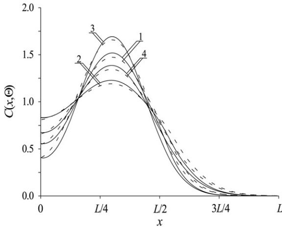
**Fig. 2.** Calculated distribution of dopant after annealing with continuance  $\Theta = 0.0025D_{0L}/L^2$  (curves 1 and 3) and  $\Theta = 0.005D_{0L}/L^2$  (curves 2 and 4). Curves 1 and 2 are correspond to spatial of distribution of dopant in homogeneous material. Curves 3 and 4 are correspond to spatial distribution of dopant in MS for  $D_2 < D_1$  and  $D_1/D_2 = 4$ . Solid lines are analytical results. Dashed lines are numerical results. Coordinate of interface is equal to  $a = L/2$ .
