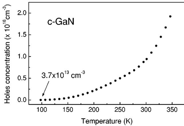
FIG. 1. The concentration of holes in terms of the lattice temperature in c-GaN in the experimental conditions of Ref. 12.
