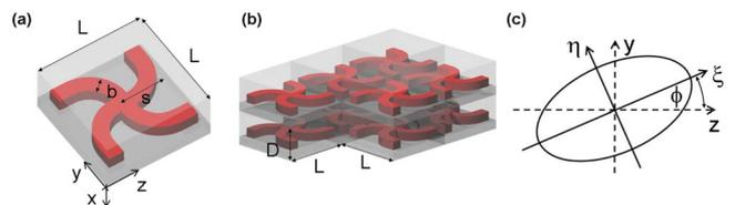
FIG. 1. (Color online) Schematics of the unit cells. (a) Metallic gammadion on substrate embedded in dielectric. (b) Sketch of the periodic arrangement. (c) The polarization ellipse along with the definition of relevant qualities.
