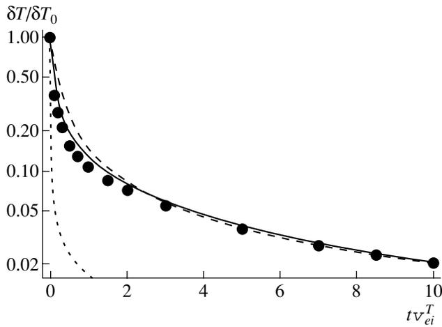
**Fig. 3.** Time evolution of the temperature at the center of a hot spot for  $Z = 10$  (circles) in the case of a thermal perturbation with an initial scale length of  $L/\lambda_{ei} = 0.1$  and the corresponding results from quasistatic theory (dashed curve) and classical theory of a strongly collisional plasma (dotted curve). The solid curve represents the temperature calculated from approximate formula (24).
