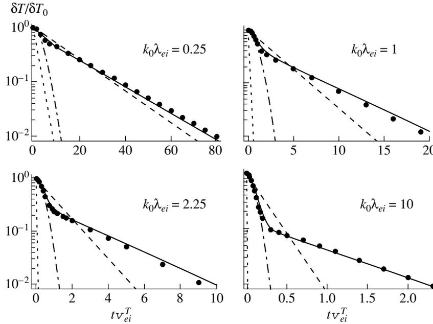
**Fig. 1.** Time evolution of periodic temperature perturbations at different initial spatial scales  $k_0$  (circles) for  $Z = 10$  and the corresponding results from quasistatic theory (dashed curves), classical collisional theory (dotted curves), and collisionless approximation (dashed-and-dotted curves). The solid curves were calculated from approximate formula (24).
