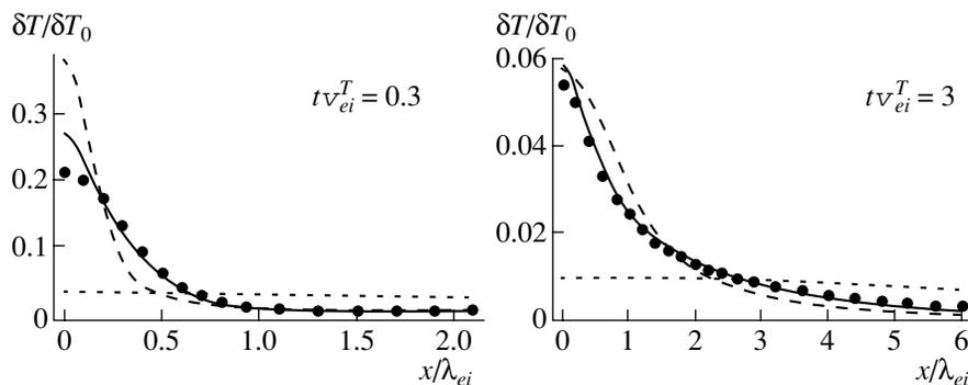
**Fig. 4.** Spatial temperature profiles for  $Z = 10$  (closed circles) in the case of a thermal perturbation with an initial scale length of  $L/\lambda_{ei} = 0.1$  and the corresponding results from quasistatic theory (dashed curves) and classical theory of a strongly collisional plasma (dotted curves). The solid curves represent the temperature calculated from approximate formula (24).
