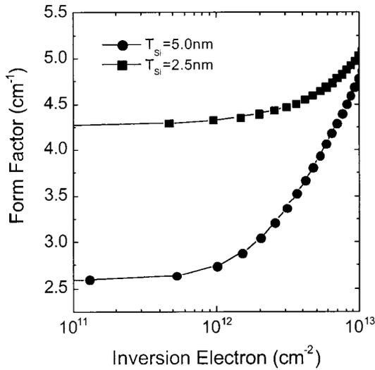
FIG. 9. Form factor for the ground subband of strained-Si/SiGe-OI inversion layers with different values of strained-Si layer thickness,  $T_{Si}$ . ( $x = 0.3$ ,  $T_w = 10$  nm).
