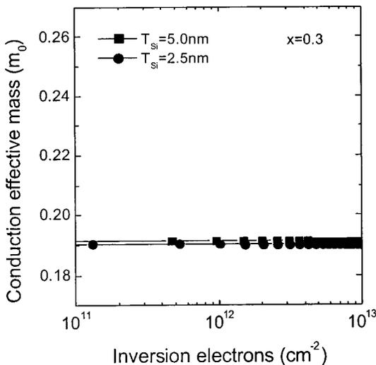
FIG. 10. Conduction effective mass of electrons in strained-Si/SiGe-OI inversion layers with different values of strained-Si layer thickness,  $T_{Si}$ . ( $x = 0.3$ ,  $T_w = 10$  nm).
