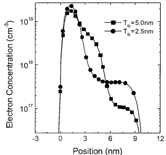
FIG. 8. Electron distribution for the simulated strained Si/SiGe-OI structure of Fig. 1 for different values of silicon layer thickness,  $T_{Si}$ . ( $x = 0.3$ ,  $T_w = 10$  nm,  $N_{inv} = 4.0 \times 10^{12}$  cm $^{-2}$ ).
