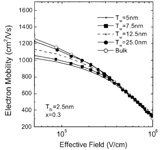
FIG. 14. Electron mobility curves versus the transverse effective field for strained Si/SiGe-OI inversion layers at room temperature for different values of  $T_w$ . ( $x = 0.3$ ,  $T_{Si} = 2.5$  nm).
