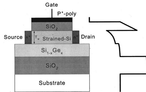
FIG. 1. Cross section of the strained-Si/SiGe-OI inversion layer under study. (Gate oxide thickness  $T_{ox} = 5$  nm, buried oxide thickness  $T_{box} = 80$  nm).
