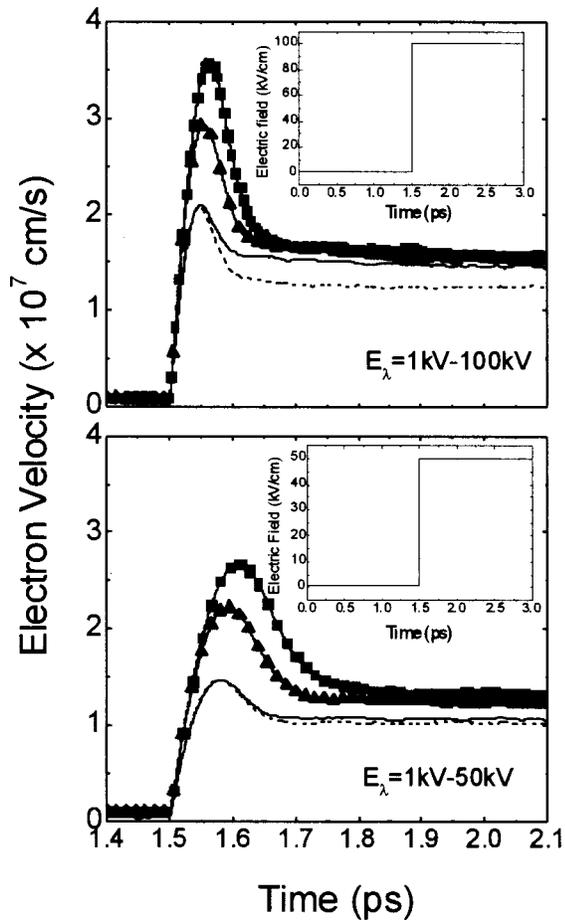
FIG. 15. Electron velocity overshoot transient resulting from the sudden application of a drift electric field  $E_2$  for different values of the germanium mole fraction (triangles:  $x=0.15$ ; squares:  $x=0.3$ ) in strained Si/SiGe-OI inversion layers ( $T_{\text{Si}}=5$  nm,  $T_w=10$  nm,  $x=0.3$ ) and in an unstrained SOI inversion layer (dashed line:  $T_{\text{Si}}=5$  nm; solid line:  $T_{\text{Si}}=10$  nm).
