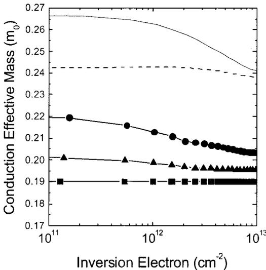
FIG. 4. (symbols) Conduction effective mass of electrons of strained-Si/SiGe-OI inversion layers with different values of the germanium mole fraction,  $x$ : circles:  $x=0.1$ ; triangles:  $x=0.15$ ; squares:  $x=0.3$ . ( $T_{Si}=T_{SiGe}=5$  nm). For the sake of comparison, the conduction effective mass of electrons in unstrained SOI inversion layers is shown without symbols: dashed line:  $T_{Si}=T_w=5$  nm; solid line:  $T_{Si}=T_w=10$  nm.
