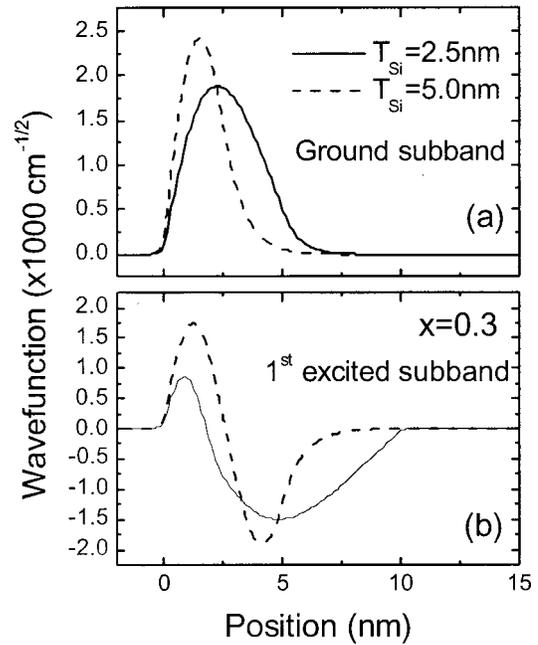
FIG. 7. (a) Wave functions for the ground subband and (b) for the first excited subband in a strained-Si/SiGe-OI inversion layer for two values of  $T_{Si}$ . ( $T_w = 10$  nm,  $x = 0.3$ ).
