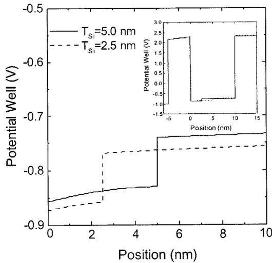
FIG. 6. Detail of the discontinuity of the conduction band minimum at the Si/SiGe interface of a strained-Si/SiGe-OI for two values of the strained silicon layer thickness ( $T_w = 10$  nm,  $x = 0.3$ ). (inset) Potential well for a strained-Si/SiGe-OI inversion layer for an inversion charge concentration of  $N_{inv} = 5.3 \times 10^{11}$  cm $^{-2}$ .
