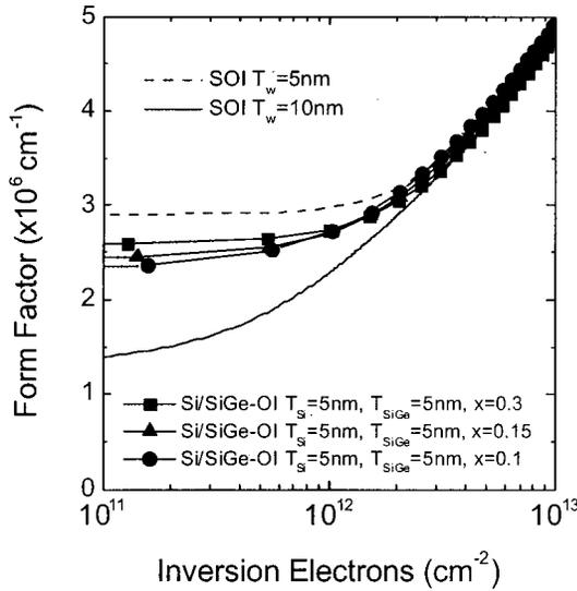
FIG. 3. (symbols) Form factor for the ground subband of strained-Si/SiGe-OI inversion layers with different values of the germanium mole fraction. (without symbols) Form factor for the ground subband of unstrained SOI inversion layers.
