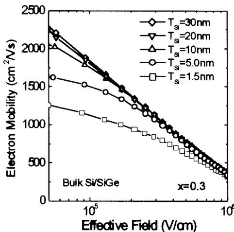
FIG. 13. Electron mobility curves versus the transverse effective field for strained Si/SiGe bulk inversion layers at room temperature for different values of  $T_{Si}$ . ( $x = 0.3$ ).
