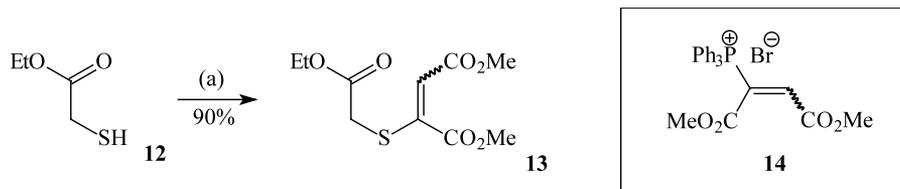
Scheme 4. (a)  $\text{PPh}_3$ , DMAD, dioxane,  $10^\circ\text{C}$ , 1 h; then reflux, 16 h.
