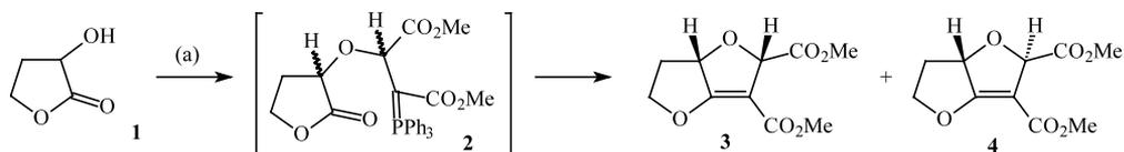
**Scheme 1.** (a) PPh<sub>3</sub>/DMAD/dioxane/10°C, 1 h, then reflux 3 h 84% (2:1).
