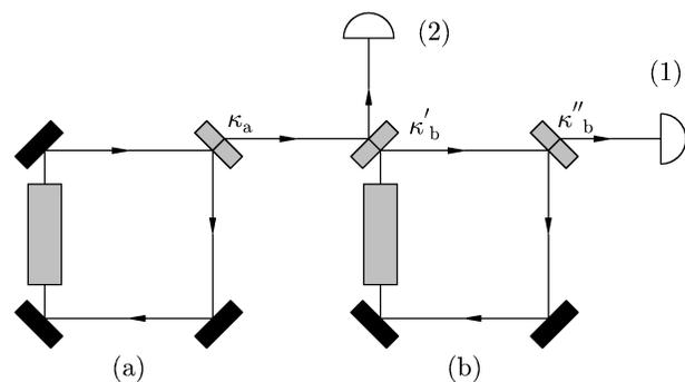
FIG. 1. The scheme of driving bistable optical resonator (b) by a sub-Poissonian laser (a) with unidirectional coupling.
