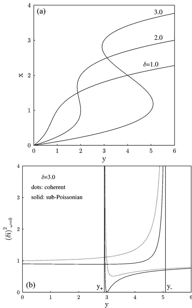
FIG. 2. (a) Bistability curve: intracavity scaled intensity  $x$  vs input intensity  $y$  for different parameters  $\delta$ ,  $\delta = 1.0, 2.0, 3.0$ ; (b) photocurrent noise spectrum at zero frequency,  $(\delta i)^2_{\omega=0}$ , for coherent (dots) and sub-Poissonian (solid) input signal,  $\delta = 3.0$ .
