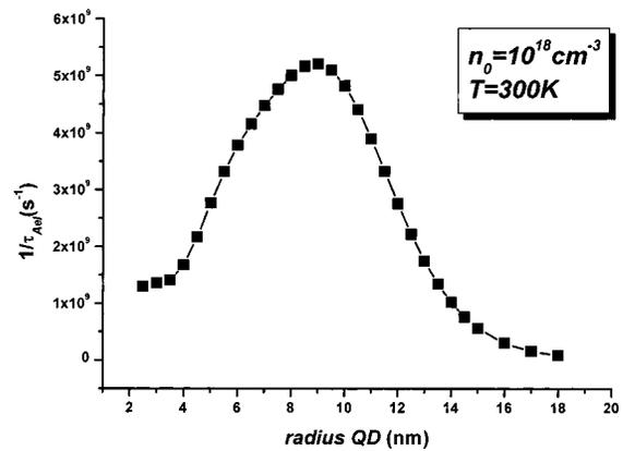
FIG. 2. Inverse time of nonradiative recombination of an electron-hole pair in a QD vs QD radius.  $T=300$  K,  $n_0=10^{18}$  cm<sup>-3</sup>.
