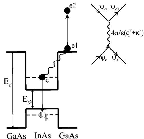
FIG. 1. Nonradiative recombination of an electron-hole pair in a QD (InAs/GaAs) via Coulomb interaction with a carrier from the barrier region.  $E_{g1} = 1.42$  eV,  $E_{g2} = 0.35$  eV. Inset: diagram describing the process.  $\Psi_e$ ,  $\Psi_h$  are the wave functions of electron and hole localized in the QD;  $\Psi_{e1}$ ,  $\Psi_{e2}$  are the initial and final wave functions of a carrier (electron or hole) from the barrier region.
