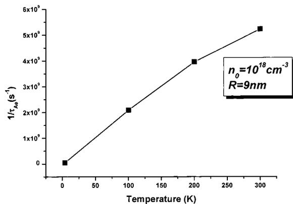
FIG. 3. Probability of nonradiative recombination of an electron-hole pair in a QD vs temperature  $T$ .  $R=9$  nm,  $n_0=10^{18}$   $cm^{-3}$ .
