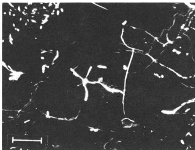
Fig. 8. Scanning electron micrograph of K_{0.4}Na_{0.6}TaO_3 ; bright areas are Na-rich (bar = 50 \mu m ).
