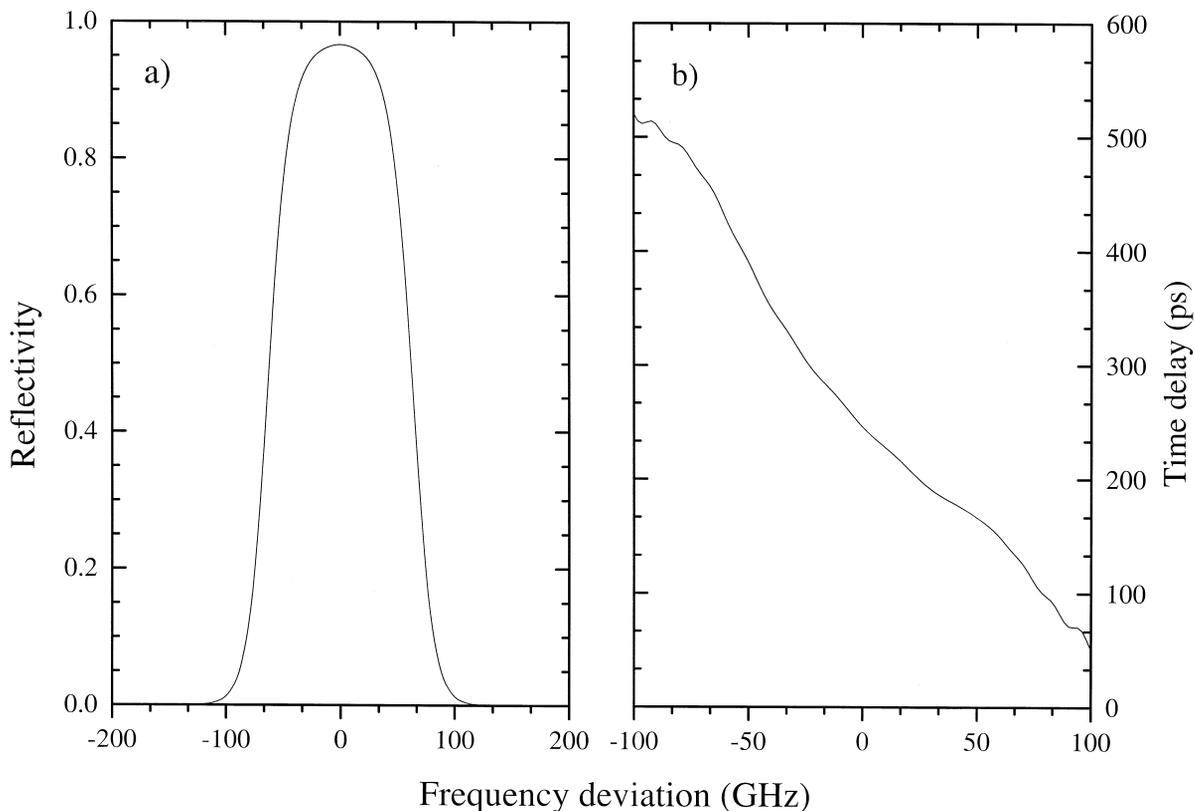
Fig. 4. Reflectivity (a) and time delay (b) of the 5.75 cm fibre Bragg grating.
