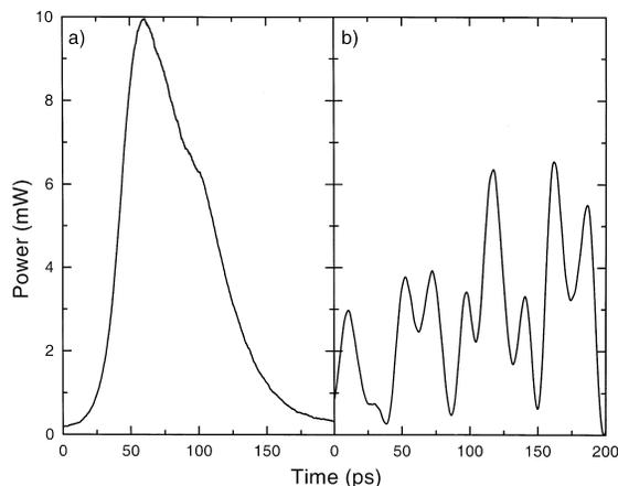
Fig. 2. (a) Isolated pulse with  $\alpha = 5$  at the laser output. (b) The same pulse after 100 km propagation.
