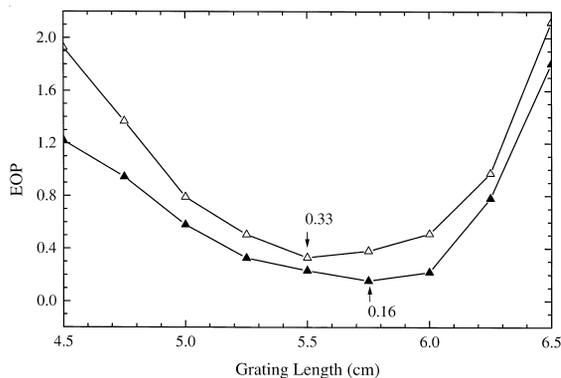
Fig. 1. Evolution of the eye-opening penalty with the grating length. Obvious differences arise between the cases of pre- (hollow triangles) and post-compensation (black triangles). The minimum EOP for the post-compensation case is 0.16, while 0.33 is achieved with pre-compensation.
