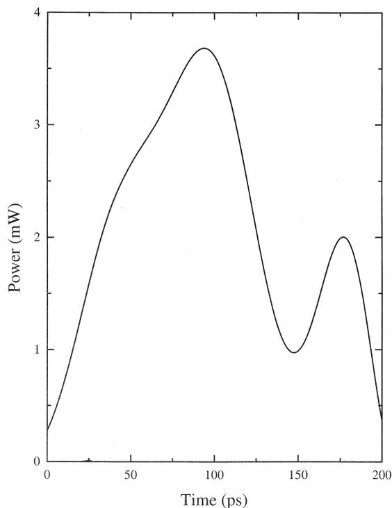
Fig. 5. Isolated chirped pulse with  $\alpha = 5$  after pre-compensation with the 5.75 cm fibre Bragg grating
