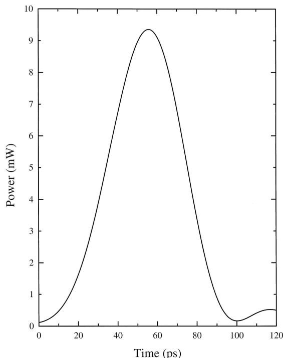
Fig. 6. Isolated chirped pulse with  $\alpha = 5$  after propagation through 100 km of SSM fibre with post-compensation.
