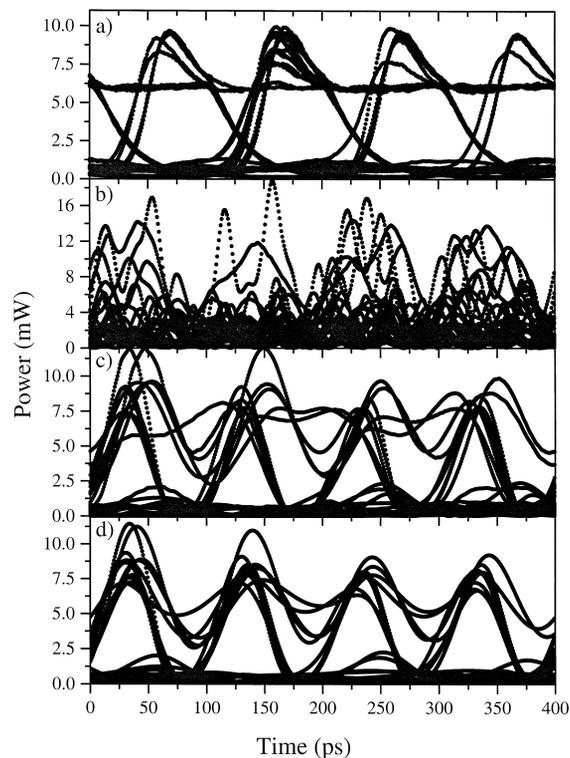
Fig. 3. Comparative eye-opening diagrams for a chirped signal with  $\alpha = 5$ . (a) Laser output. (b) After 100 km without compensation. (c) After 100 km with pre-compensation. (d) After 100 km with post-compensation.
