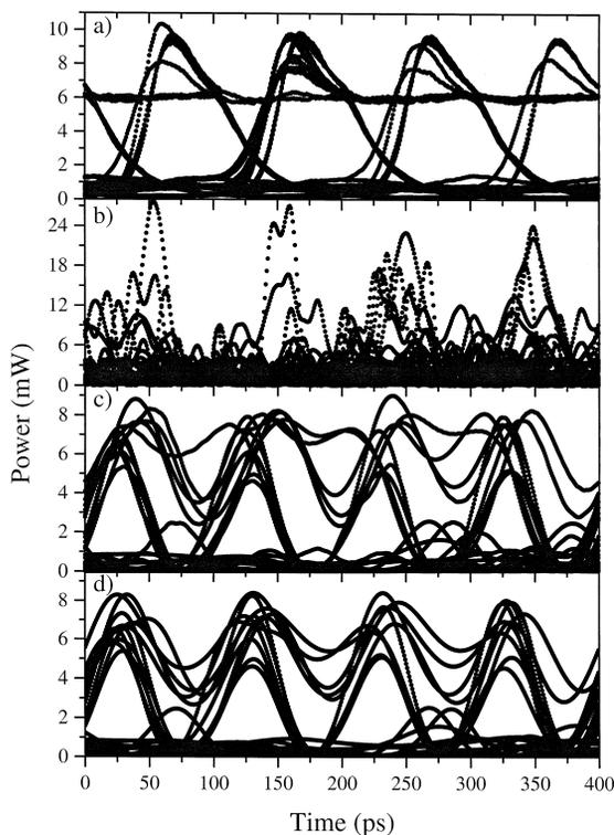
Fig. 7. Comparative eye-opening diagrams for a chirped signal with  $\alpha = 8$ . (a) Laser output. (b) After 100 km without compensation. (c) After 100 km with pre-compensation. (d) After 100 km with post-compensation.
