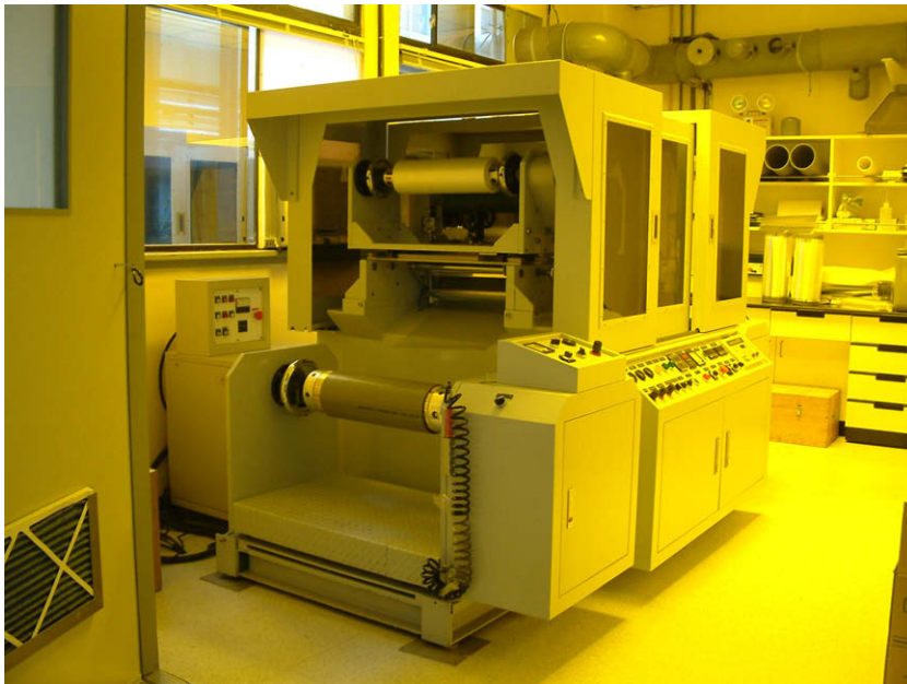
Fig. 7. Picture of the roller imprinting equipment designed by ITRI for continuous nanostructure duplication.
