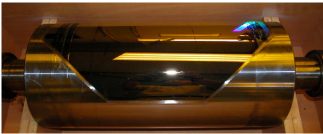
Fig. 6. Picture of the bonded roller mold adhered with ASS Ni mold.
