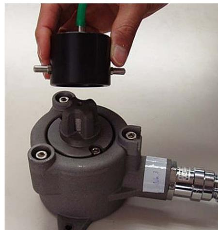
**Fig. 8 – Photo of the sensing performance test using the pressure proof enclosure with gas flow of 1 L/min.**
