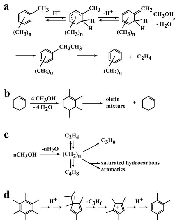
**FIGURE 4.** Early proposals that have significantly shaped current thinking about the hydrocarbon pool mechanism in MTO catalysis. (a) Mole's 1983 mechanism of methylbenzene side-chain alkylation. (b) An abbreviated account of Langner's explanation for the dramatic effect of cyclohexanol and other co-feeds of reducing the kinetic induction period. (c) Kolboe's early phenomenological hydrocarbon pool mechanism for MTO catalysis. (d) The paring reaction in highly abbreviated form.
