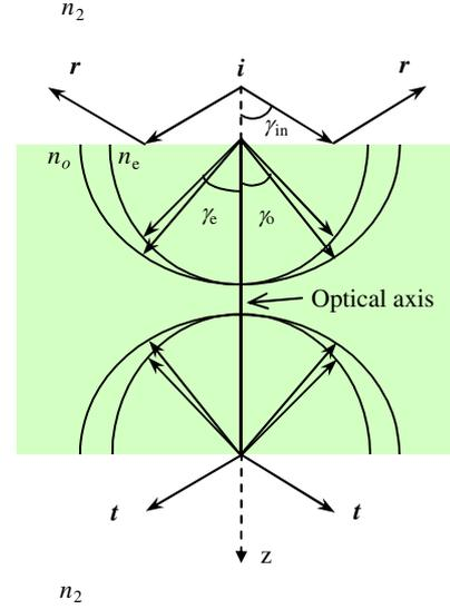
Fig. 2. Transmission of Bessel beam through the layer of uniaxial crystal.  $i$ ,  $r$  and  $t$  designate input, reflected and transmitted Bessel beams.
