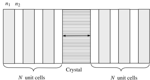
Fig. 3. Layered-periodic medium with the defect inclusion of uniaxial crystal. The orientation of the optical crystal axis is shown by arrow.
