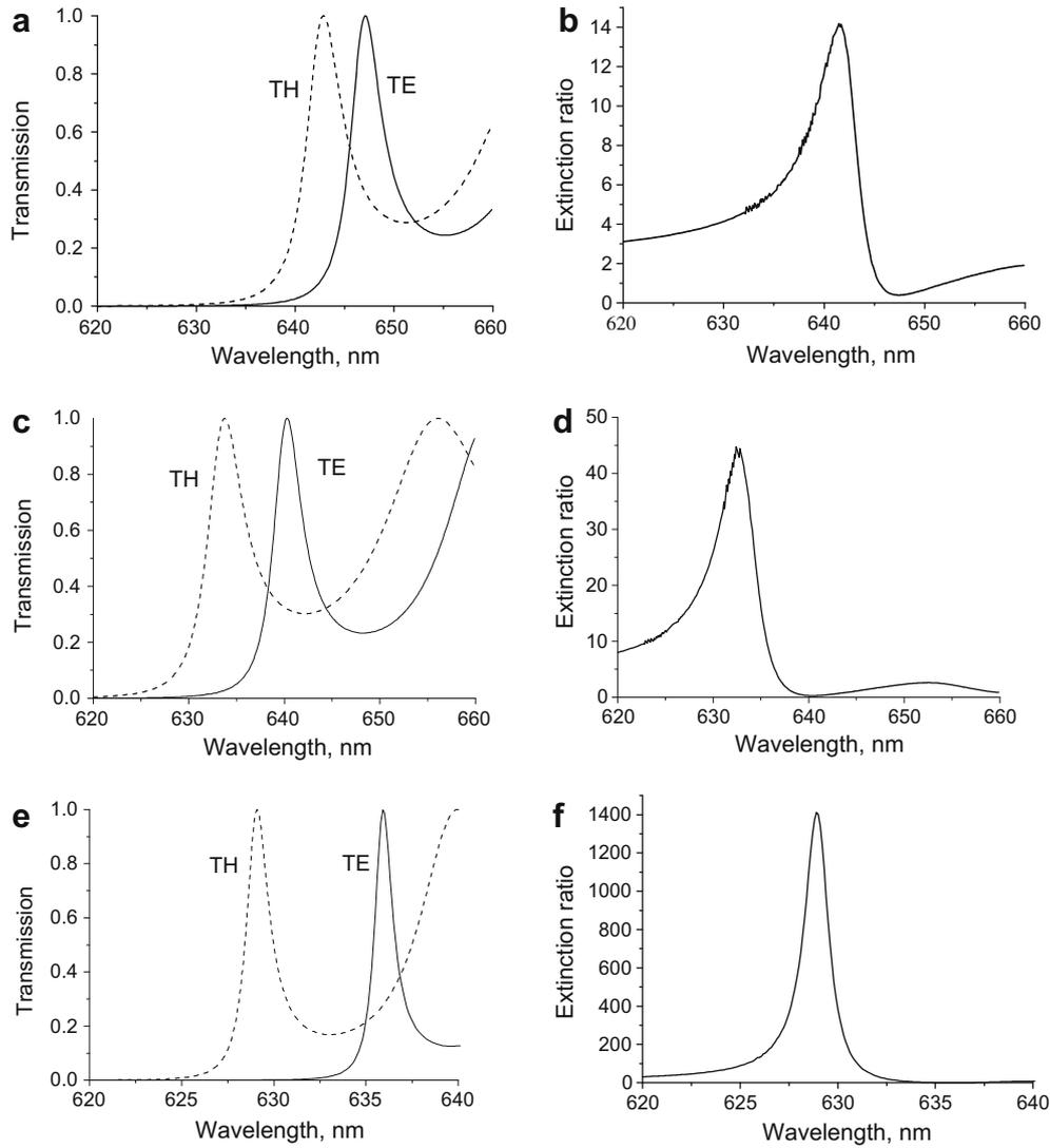
**Fig. 4.** Spectral dependence of the transmission  $\tilde{T} = |t|^2$  and extinction ratio of perfect 1DPC  $[\text{ZrO}_2/\text{SiO}_2]^N$ , containing  $N = 20$  (a–d) or  $N = 30$  (e, f) unit cells, for incident BLB having half-cone angle  $20^\circ$  (a, b) or  $25^\circ$  (c–f).
