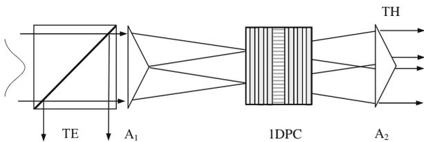
**Fig. 8.** Optical scheme for formation of TE- and TH-polarized BLBs.  $A_{1,2}$  are axicons; 1DPC is a one-dimensional photonic crystal (perfect of having a crystalline defect layer).
