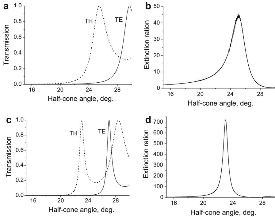
**Fig. 5.** Angle dependence of transmission  $\tilde{T} = |t|^2$  and extinction ratio of perfect 1DPC  $[\text{ZrO}_2/\text{SiO}_2]^N$ , containing  $N = 20$  (a, b) or  $N = 30$  (c, d) unit cells, for incident BLB having wavelength  $\lambda = 0.6328 \mu\text{m}$ .
