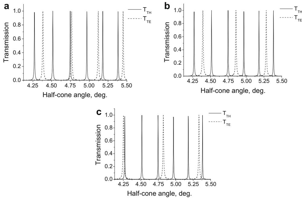
**Fig. 7.** Dependences of transmission  $\tilde{T} = |t_s|^2$  of  $[\text{ZrO}_2/\text{SiO}_2]^5/\text{anisotropy layer}/[\text{ZrO}_2/\text{SiO}_2]^5$  structure on the half-cone angle of incident BLB having wavelength  $\lambda = 0.6328 \mu\text{m}$ . Parameters:  $d_{1,2} = \lambda/4n_{1,2}$ . The principle refractive indices of model anisotropy layer are  $n_o = 1.85$  (a), 2.05 (b), 2.25 (c);  $n_e = 1.45$ .
