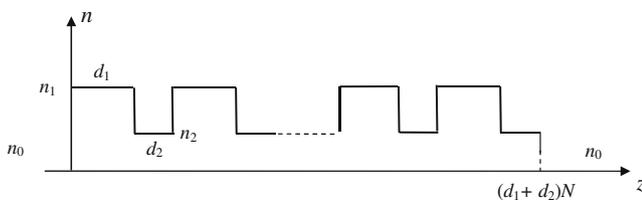
**Fig. 1.** Example: one-dimensional photonic crystal with a  $N$ -period stack composed of two-layer unit cells of thickness  $d_1$  and  $d_2$  and refractive indices  $n_1$  and  $n_2$ , respectively.
