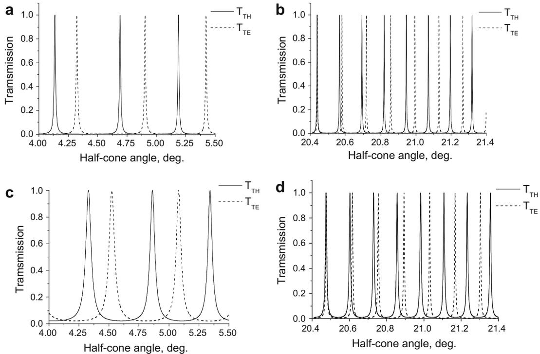
**Fig. 6.** Dependences of transmission  $\tilde{T} = |t_s|^2$  of  $[\text{ZrO}_2/\text{SiO}_2]^5/\text{LiNbO}_3/[\text{ZrO}_2/\text{SiO}_2]^5$  structure on half-cone angle of incident BLB having the wavelength  $\lambda = 0.6328 \mu\text{m}$ . Parameters:  $d_{1,2} = \lambda/4n_{1,2}$  (a, b);  $d_{1,2} = 1.12\lambda/4n_{1,2}$  (c, d). The principle refractive indices of  $\text{LiNbO}_3$  are  $n_o = 2.2878$  and  $n_e = 2.1890$ .
