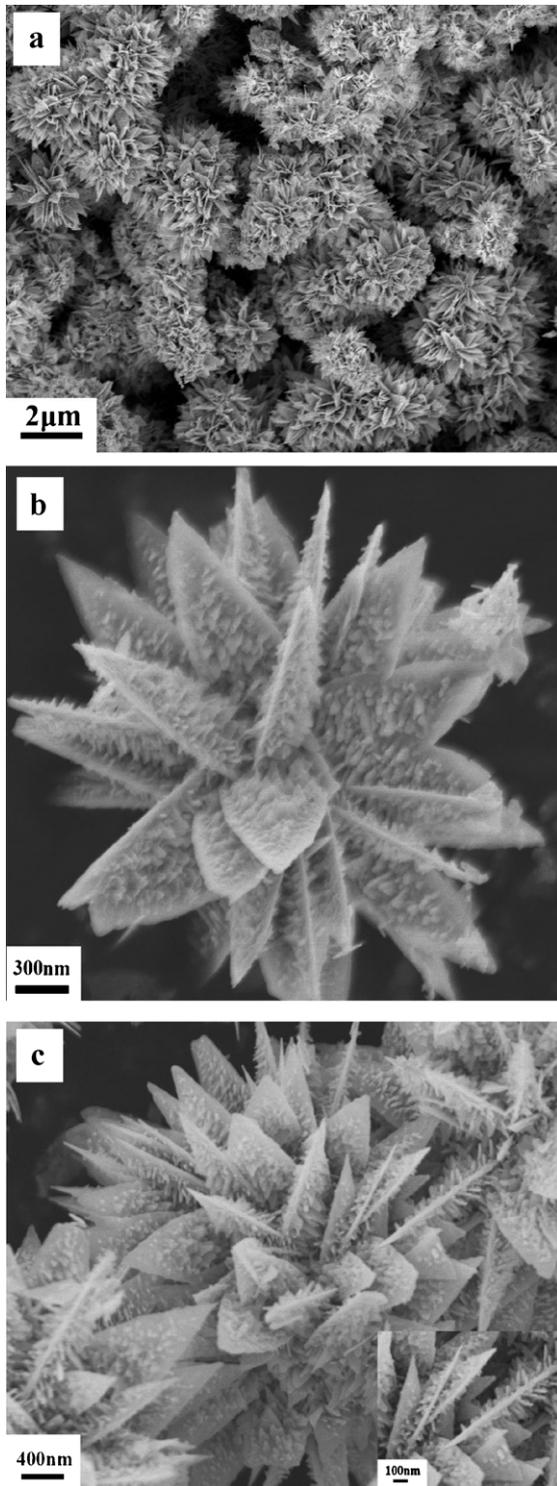
Fig. 3. Low and high-magnification SEM images of aloe-like SnO<sub>2</sub> nanostructures obtained at 550 °C.
