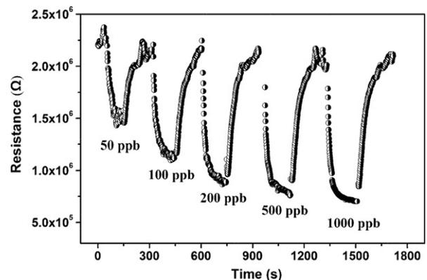
Fig. 6. Real time response of aloe-like SnO<sub>2</sub> nanostructures to ethanol with concentrations in the range of 50–1000 ppb at 285 °C.
