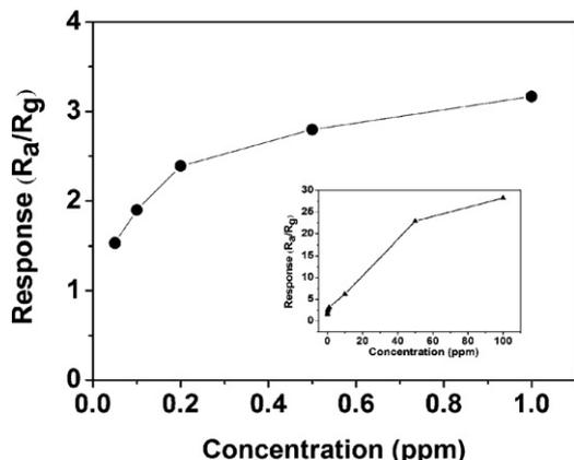
**Fig. 7.** Response of aloe-like SnO<sub>2</sub> nanostructures to various concentrations of ethanol at 285 °C.
