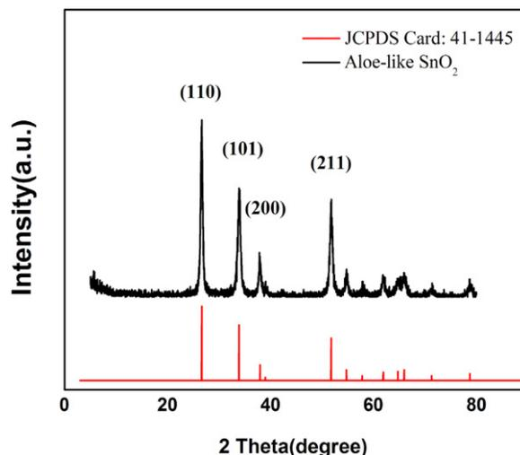
Fig. 2. XRD patterns of aloe-like SnO<sub>2</sub> nanostructures obtained at 550 °C.
