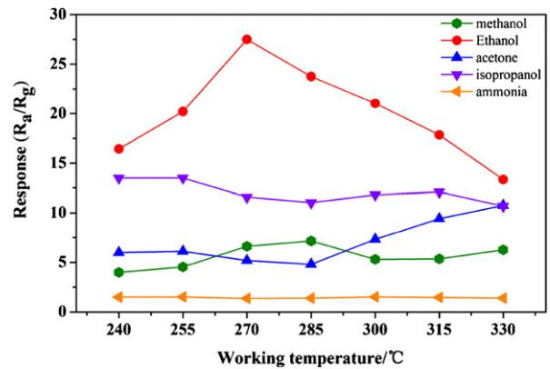
Fig. 4. The response of aloe-like SnO<sub>2</sub> nanostructures based sensor to 50 ppm ethanol, methanol, acetone, isopropanol and ammonia at different working temperatures.
