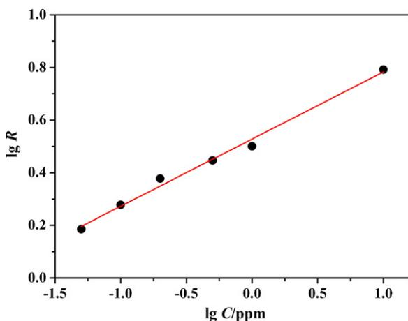
**Fig. 8.** The relationship between the sensor response and the ethanol concentration.
