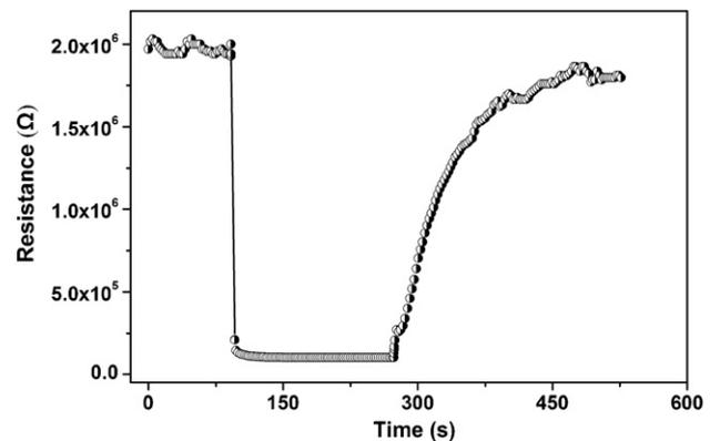
Fig. 5. Real time response of aloe-like SnO<sub>2</sub> nanostructures to 50 ppm ethanol at a working temperature of 285 °C.
