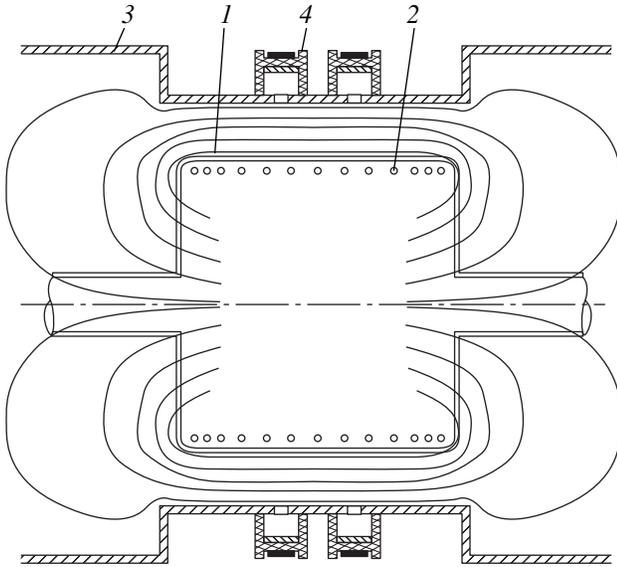
**Fig. 8.** Configuration of the magnetic field in one of the six units of the MOL facility: (1) POS anode with magnetic-field coils inside it, (2) one turn of the magnetic-field coil, (3) POS cathode, and (4) plasma injectors.
