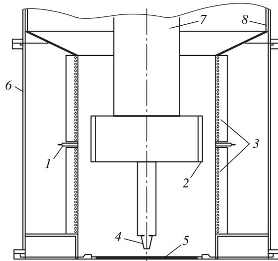
**Fig. 7.** Schematic of the POS of the UIN-10 accelerator: (1) one of 48 plasma injectors, (2) POS cathode, (3) 600-mm-diameter 380-mm-long magnetic-field coils, (4) cathode of the electron diode, (5) X-ray anode-converter of the electron diode, (6) outer surface of the vacuum chamber, (7) MITL cathode, and (8) MITL anode.
