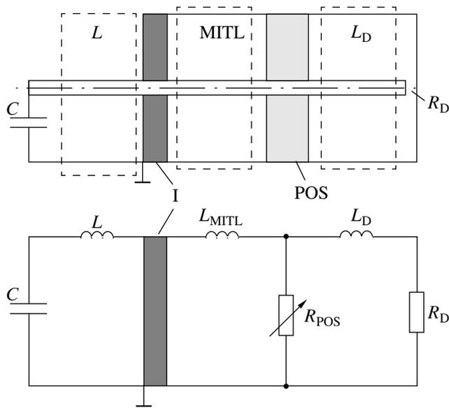
**Fig. 1.** Electric circuit of a high-power pulsed generator with a POS for the sharpening of the power of the inductive energy storage: (C) primary capacitive energy storage (Marx generator), (L) inductance of the input circuit, (I) high-voltage vacuum insulator, ( $L_{MITL}$ ) inductance of the MITL, ( $R_{POS}$ ) plasma bridge of the POS with a nonlinear impedance, ( $L_D$ ) inductance of the line transferring energy into the load, and ( $R_D$ ) load (e.g., an electron diode).
