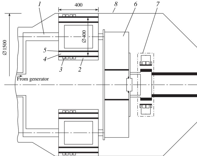
**Fig. 9.** Axial cross section of the load of the MOL facility with six POSs connected in parallel: (1) current lead (anode), (2) POS cathode, (3) plasma injectors, (4) anode-cathode gap of the POS, (5) POS anode with magnetic-field coils, (6) spark gap, (7) POS (plasma bridge) for simulating a load with a nonlinear impedance, and (8) vacuum chamber.
