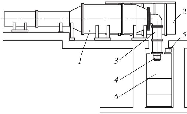
**Fig. 5.** Schematic of the UIN-10 accelerator with a POS: (1) capacitive energy storage (Marx generator), (2) protective screen, (3) MITL, (4) POS, (5) capacitor bank for powering the plasma injectors of the POS, and (6) research chamber.
