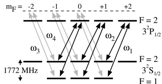
FIG. 1. Transition scheme within the Na  $D_1$  line for  $\Lambda$  (black) and double- $\Lambda$  excitation (black and gray).
