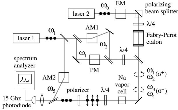
FIG. 2. Experimental setup. EM: electro-optical modulator, AM1/2: acousto-optical modulator, PM: phase modulator.
