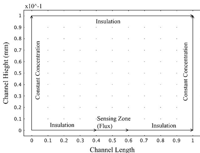
FIGURE 2 Two-dimensional channel design with the boundary conditions for each wall.
