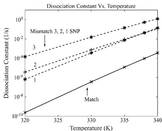
FIGURE 3 Dissociation rate constants at different temperatures for the match (solid line), and a 3-, 2-, or 1-SNP mismatch target (dashed line).
