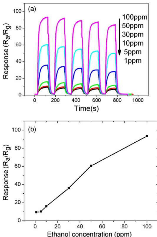
**Fig. 4.** (a) Sensitivity response vs. time for ethanol concentrations of 1–100 ppm at a work temperature of 300 °C. (b) Sensor response vs. ethanol concentration.
