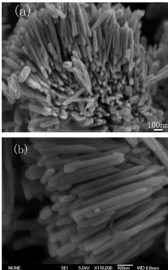
Fig. 2. (a) Low- and (b) high-magnification SEM images of ZnO nanorods.
