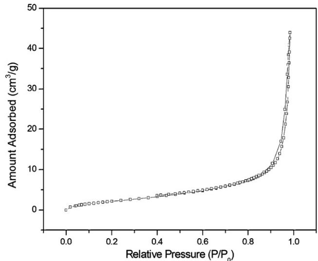
Fig. 3.  $N_2$  adsorption/desorption isotherms of ZnO nanorods.
