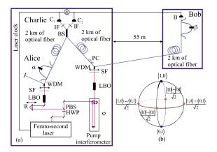
FIG. 2 (color online). (a) Long distance quantum teleportation experiment, with 2 km of optical fibers inserted between each source and the BSM. (b) Poincaré sphere representing the qubit states.
