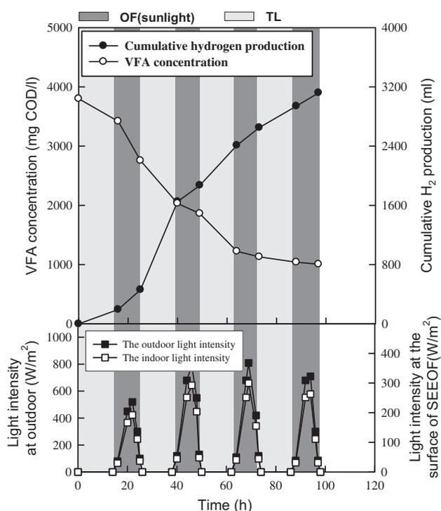
**Fig. 4 – Effect of solar-energy-excited optical fiber photobioreactor (SEEOF) on the performance of phototrophic H<sub>2</sub> production under batch operations (Dilution ratio from dark-fermented broth:1:2; Light source: OF(sunlight)/TL, where TL represents tungsten filament lamp and OF(sunlight) represents side light optical fiber excited by sunlight; added glutamic acid and yeast extract concentration was 400 and 200 mg/l, respectively).**
