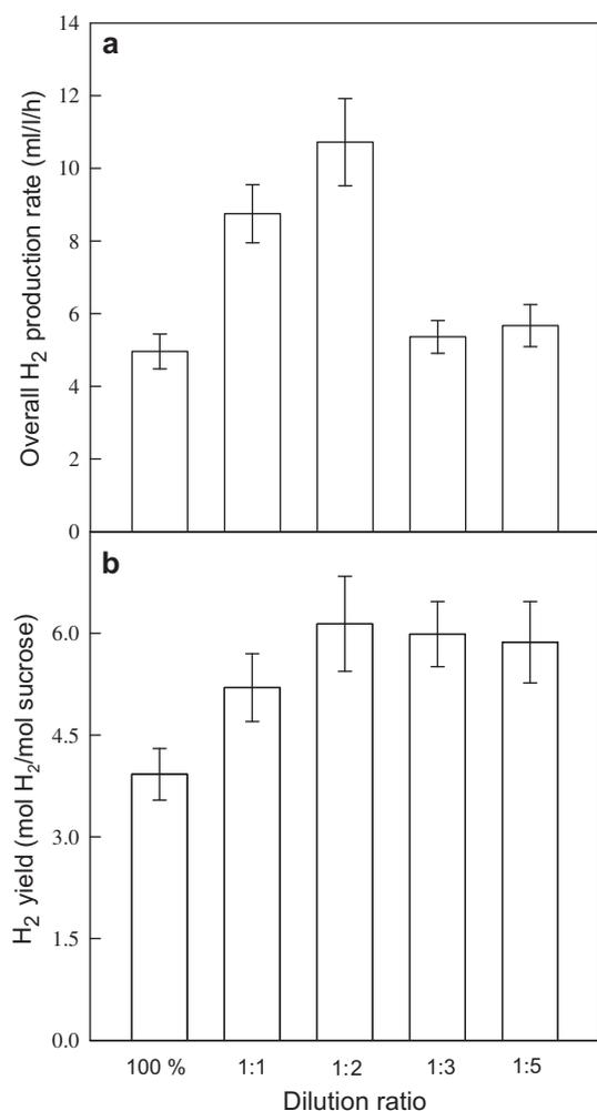
**Fig. 2 – Effect of dilution ratio on the performance of phototrophic H<sub>2</sub> production under batch operations (a) overall H<sub>2</sub> production rate and (b) H<sub>2</sub> yield. (Light source: halogen and tungsten lamp (HL/TL); total light intensity = 95 W/m<sup>2</sup>).**
