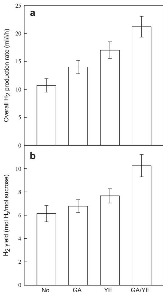
**Fig. 3** – Effect of nutrient addition on the performance of phototrophic H<sub>2</sub> production under batch operations (a) overall H<sub>2</sub> production rate and (b) H<sub>2</sub> yield. (Added concentration of glutamic acid = 400 mg/l; added concentration of yeast extract = 200 mg/l; dilution ratio for dark fermentation broth = 1:2; Light source: halogen and tungsten lamp (HL/TL); total light intensity = 95 W/m<sup>2</sup>).
