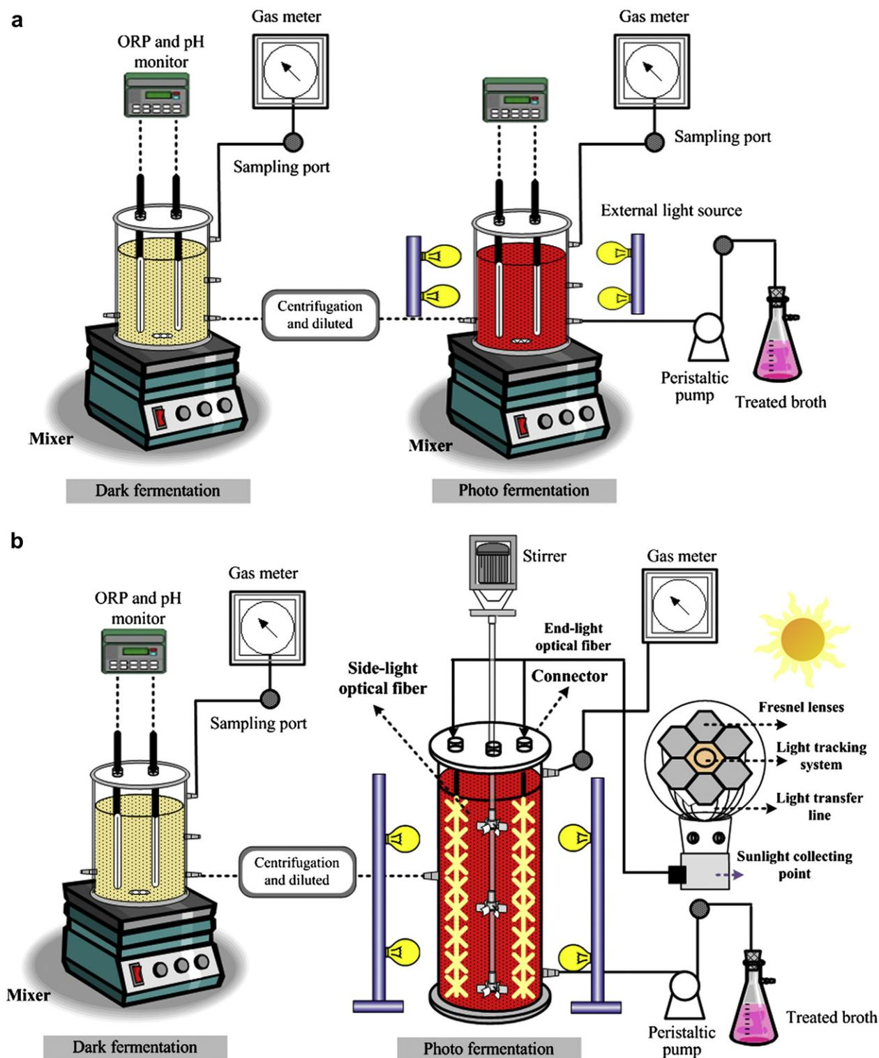
**Fig. 1 – Schematic description of the two-stage process combining dark and photo fermentation equipped with (a) only external light sources and (b) combinative internal (optical fiber excited by sunlight collecting system) and external (four tungsten filament lamp) light sources.**
