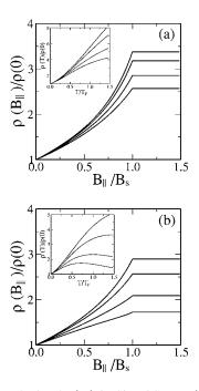
FIG. 1. The calculated  $\rho(B_{\parallel})$  in Si MOSFETs (a) for ideal 2D system and (b) for quasi-2D system at T=0 and for various densities  $n=1.0, 2.0, 5.0, 10.0 \times 10^{11}$  cm<sup>-2</sup> (from top to bottom). The insets show  $\rho(T)$  at  $B_{\parallel}=0$  and for the same systems as the main figures.
