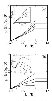
FIG. 2. The calculated  $\rho(B_{\parallel})$  in *n*-GaAs (a) for ideal 2D system and (b) for quasi-2D system at T=0 and for various densities  $n=0.4, 0.8, 1.2, 2.0 \times 10^{10}$  cm<sup>-2</sup>, (from top to bottom). The insets show  $\rho(T)$  at  $B_{\parallel}=0$  and for the same systems as the main figures.
