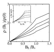
FIG. 4. The main figure (inset) shows the calculated  $\rho(B_{\parallel})$  in the realistic quasi-2D *n*-GaAs (Si MOS) system including both magneto-spin-polarization and magneto-orbital effects for various densities  $n=0.4, 0.8, 1.2, 2.0 \times 10^{10} \text{ cm}^{-2}$   $(n=1.0, 2.0, 5.0, 10.0 \times 10^{11} \text{ cm}^{-2})$ , from top to bottom.
