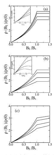
FIG. 5. The calculated  $\rho(B_{\parallel})$  in *p*-GaAs (a) for ideal 2D system and (b) for quasi-2D system at T=0 and for various densities  $n=1.0, 2.0, 5.0, 10.0 \times 10^{10}$  cm<sup>-2</sup> (from top to bottom). The insets show  $\rho(T)$  at  $B_{\parallel}=0$  and for the same systems as the main figures. In (c) the calculated  $\rho(B_{\parallel})$  in the quasi-2D system including both magneto-spin and magneto-orbital effects is shown for the same densities given in (b).
