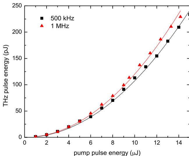
FIG. 2. (Color online) Dependence of terahertz pulse energy on the pump pulse energy at 500 kHz (squares) and 1 MHz (triangles) pump pulse repetition rates. The solid lines are the respective parabolic fits to the data.
