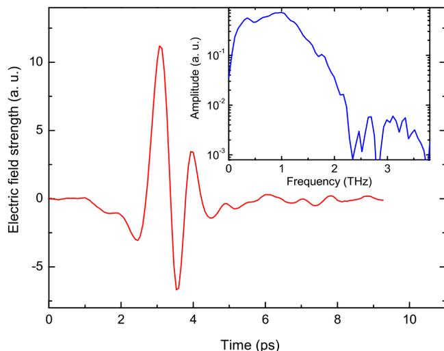
FIG. 1. (Color online) Temporal shape of the terahertz pulse generated at 1 MHz repetition rate and (inset) corresponding amplitude spectrum.
